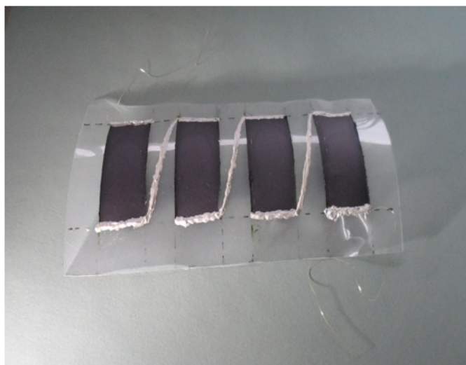
Fig. S7 Digital photograph of flexible thermoelectric module fabricated by PANI/SWNTs/Te nanocomposite films with 10 wt% Te content.
