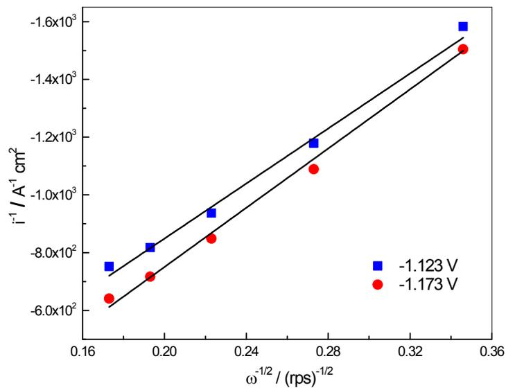
Fig. SI. 5. Koutecky-Levich plots at  $-1.123$  and  $-1.173 \text{ V}$ .
