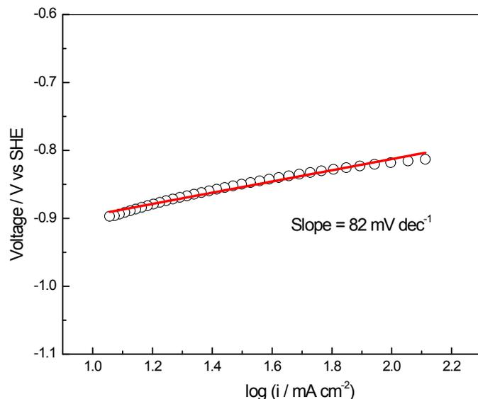
Fig. SI. 6. Tafel plot for ORR in 0.1 M TBAP-DMSO on  $Pt_3Ni$ -RGO.
