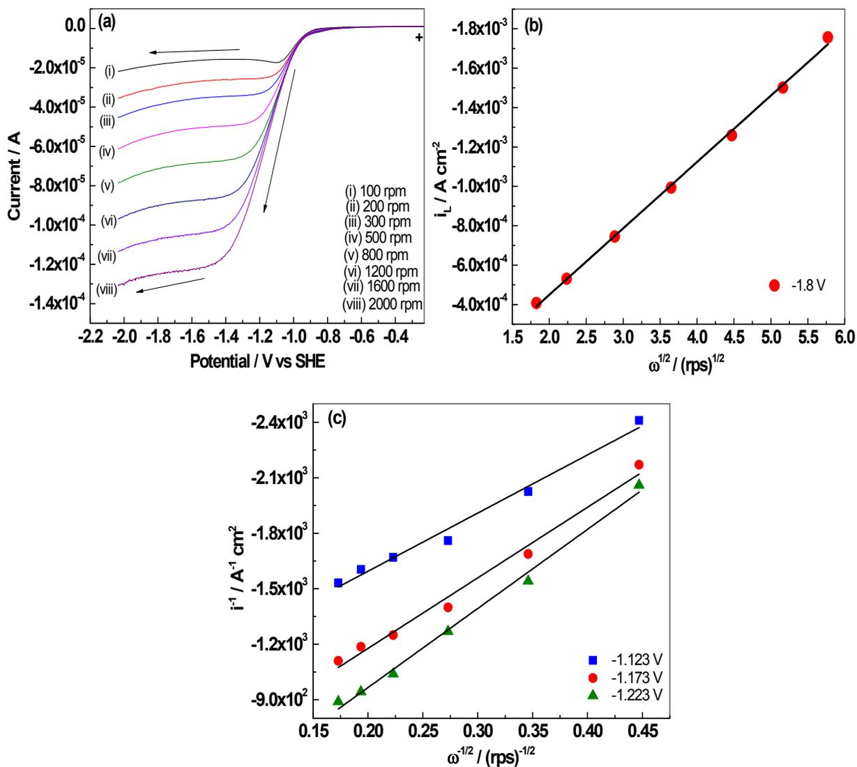
Fig. SI.8. (a) Linear sweep voltammetry of Pt-RGO coated GC electrode at  $10 \text{ mV s}^{-1}$  in O<sub>2</sub> saturated 0.1 M TBAP-DMSO at various speeds, (b) Levich plot and (c) Koutecky-Levich plot.
