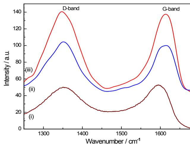
Fig. SI.1. Raman spectra of RGO (i), Pt-RGO (iii) and Pt<sub>3</sub>Ni-RGO (iv).
