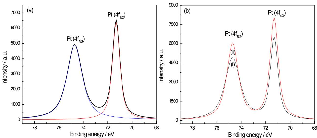
Fig. SI.2. (a) Deconvoluted XPS spectra of Pt 4f region and (b) comparison of 4f regions of Pt in Pt-RGO (i) and Pt<sub>3</sub>Ni-RGO (ii).
