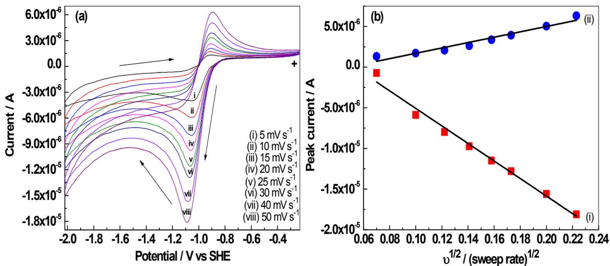
Fig. SI.7. (a) Cyclic voltammograms of Pt-RGO coated GC electrode at different scan rates and (b) plot between peak current versus  $(\text{sweep rate})^{1/2}$  for cathodic (i) and anodic peak (ii) in 0.1 M TBAP-DMSO electrolyte.
