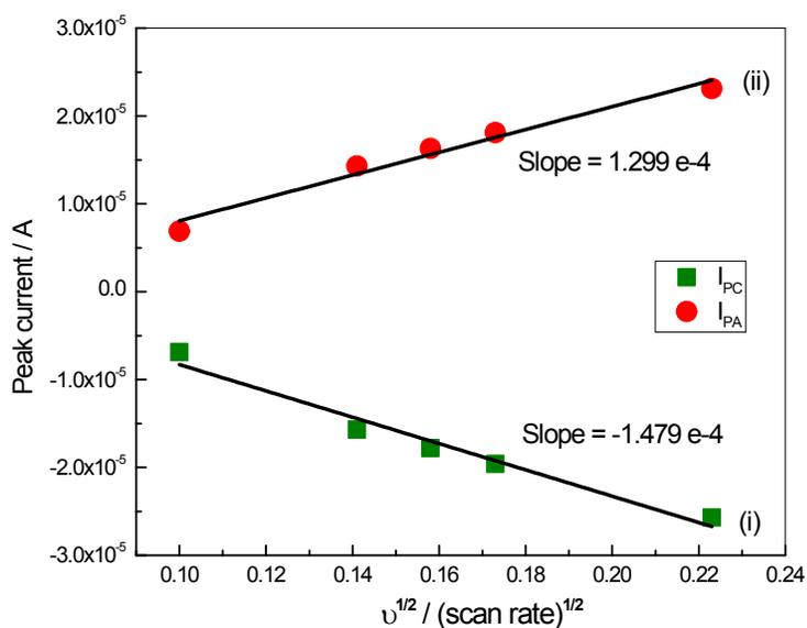
Fig. SI. 4. Plot between square root of scan rate and peak current.
