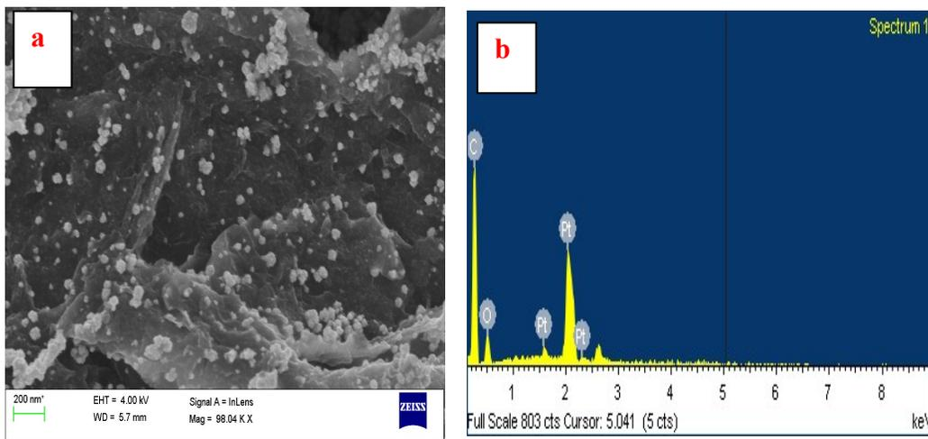
*Fig. SI.3. SEM image (a) and EDAX pattern of Pt-RGO.*
