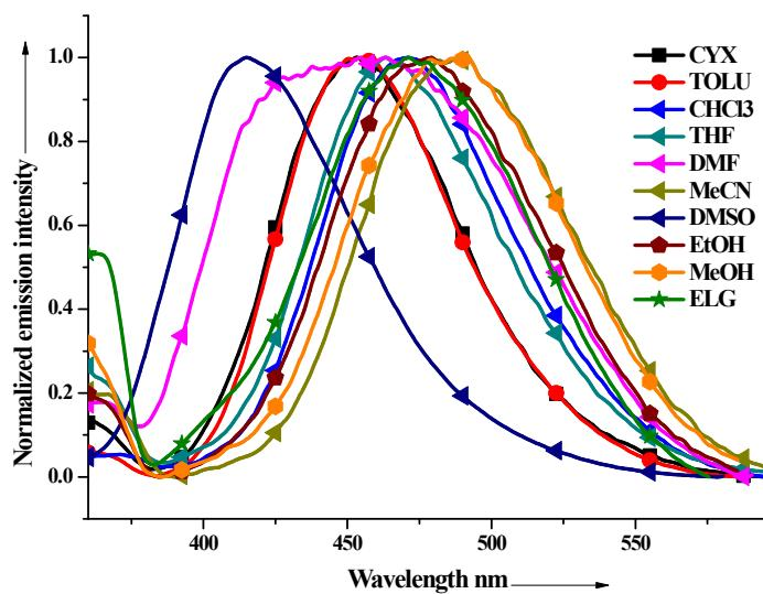
Figure S10: Emission spectra of **NIN** in different solvents.
