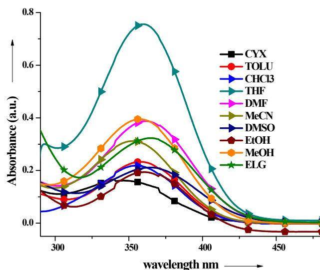
Figure S6: Absorption spectra of **NiN** in different solvents
