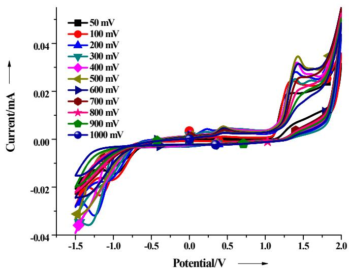
Figure S20: Cyclic volatamogram of **NIN** with multi scan rate in DMF.
