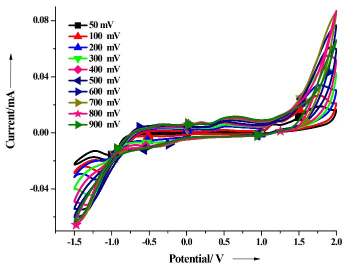
Figure S19: Cyclic volatamogram of **PYRIN** with multi scan rate in DMF.
