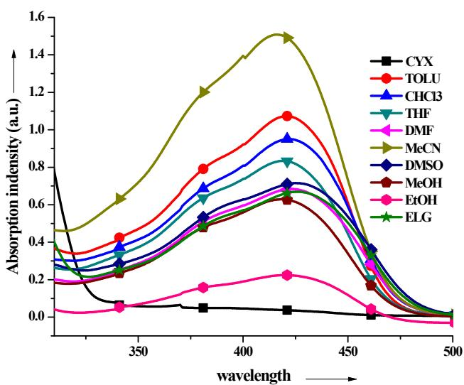
Figure S3: Absorption spectra of **T2IN** in different solvents
