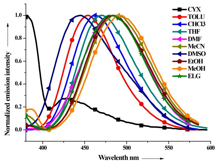
Figure S12: Emission spectra of **PY2IN** in different solvents.
