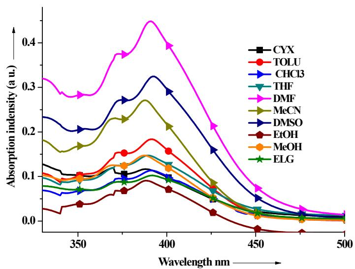
Figure S5: Absorption spectra of **AlN** in different solvents
