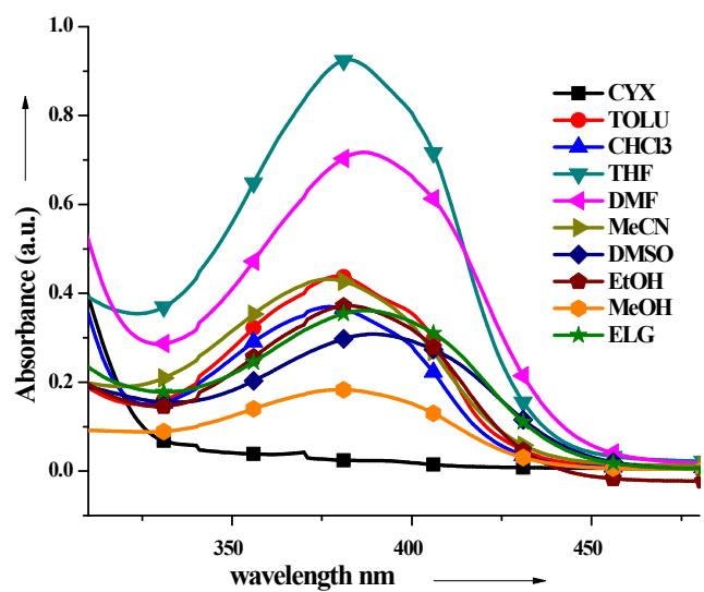
Figure S9: Absorption spectra **PY2IN** in different solvents
