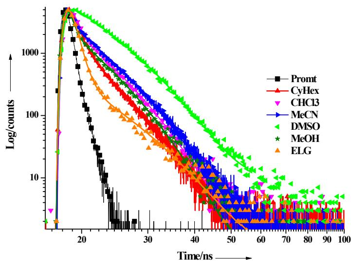
Figure S17: Fluorescence decay curves of **PYRIN** in all of the solvents studied.
