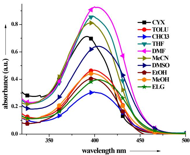
Figure S4: Absorption spectra of **TIN** in different solvents
