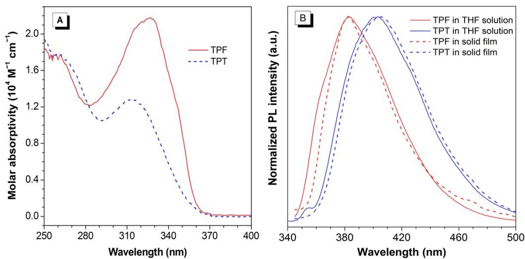
**Fig. S6** (A) UV absorption spectra of TPF and TPT in THF solutions. (B) PL spectra of TPF and TPT in THF solutions ( $10 \mu\text{M}$ ) and in solid films, excitation wavelengths: 327 nm for TPF and 320 nm for TPT.
