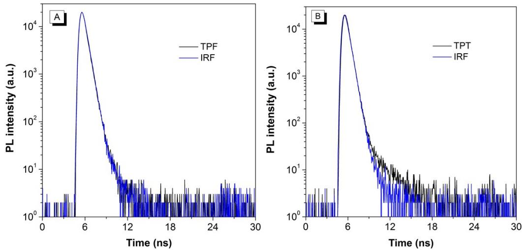
**Fig. S9** Transient PL decay curves of (A) TPF and (B) TPT in solid films, excitation wavelengths: 340 nm. Blue curves are instrument response factor (IRF) data.
