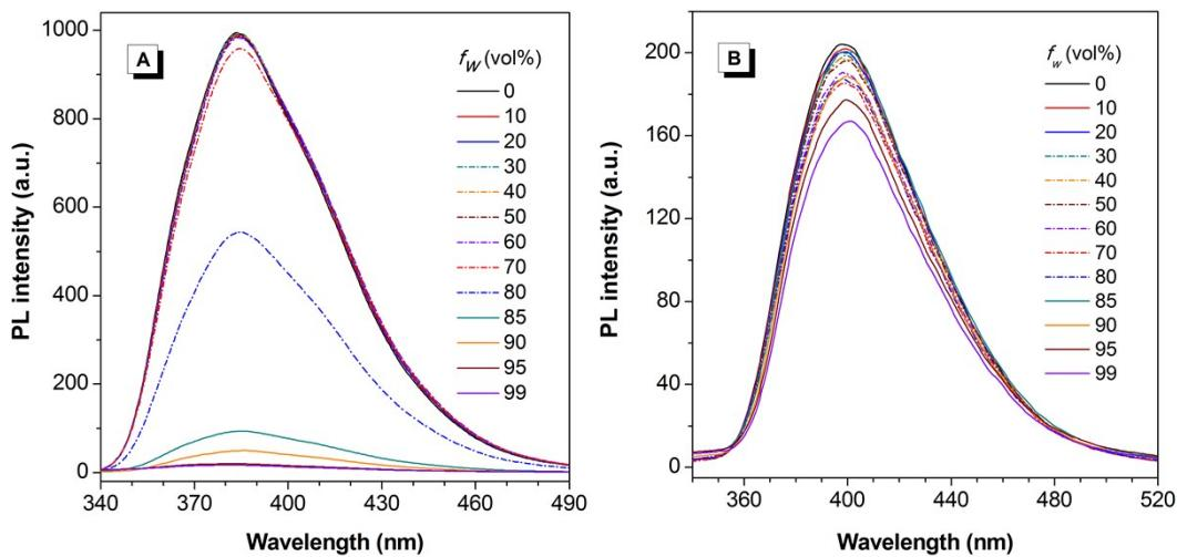
**Fig. S7** PL spectra of (A) TPF and (B) TPT in THF/water mixtures with different water fractions ( $f_w$ ). Concentration: 10  $\mu$ M; excitation wavelengths: 327 nm for TPF and 320 nm for TPT.
