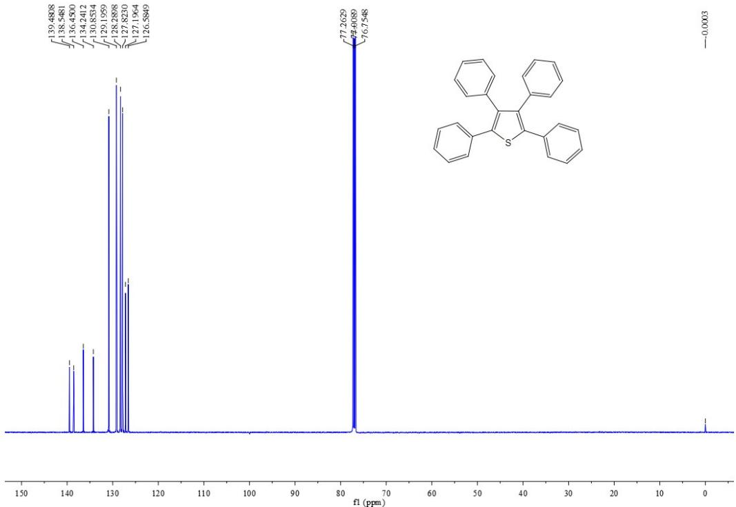
**Fig. S4**  $^{13}\text{C}$  NMR of TPT in  $\text{CDCl}_3$ .
