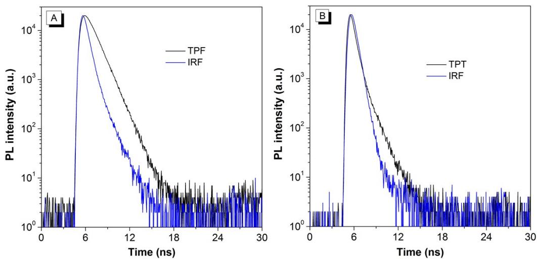
**Fig. S8** Transient PL decay curves of (A) TPF and (B) TPT in THF solutions (10  $\mu$ M). Excitation wavelengths: 340 nm. Blue curves are instrument response factor (IRF) data.
