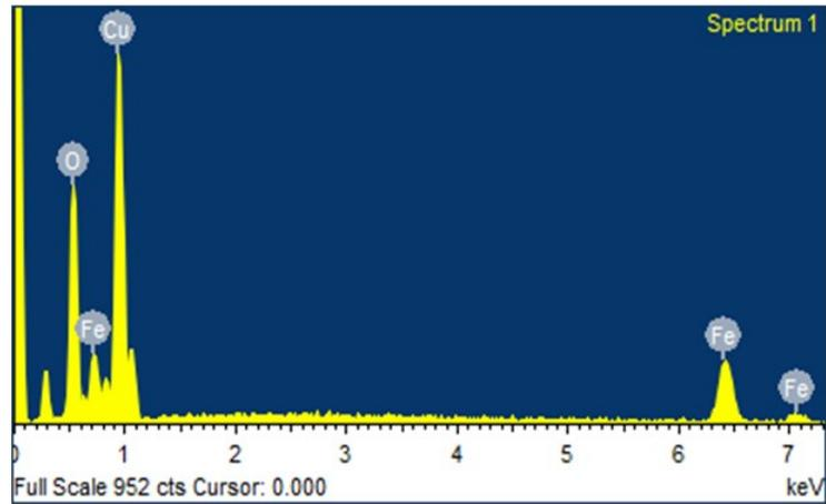
**Figure S2:** Energy dispersive X-ray spectrum of Cu(0)/Fe<sub>3</sub>O<sub>4</sub>
