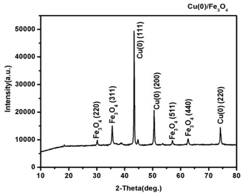
**Figure S3:** Wide angle powder X-ray diffraction pattern of Cu(0)/Fe<sub>3</sub>O<sub>4</sub>
