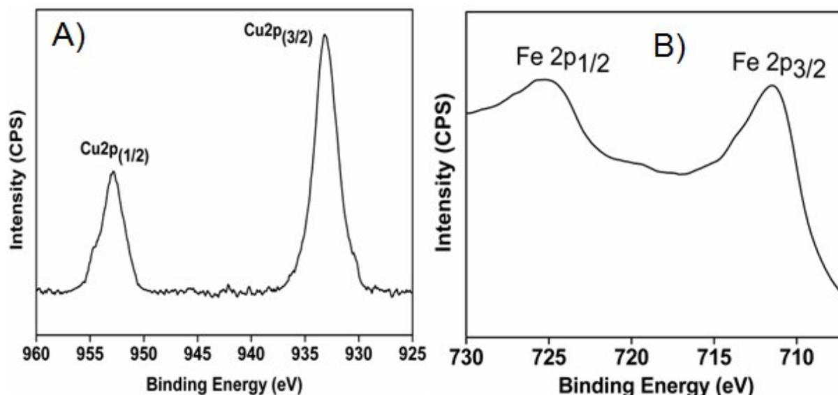
**Figure S4:** XPS spectra of Cu 2p region (A) and Fe 2p region (B) of Cu(0)/Fe<sub>3</sub>O<sub>4</sub>
