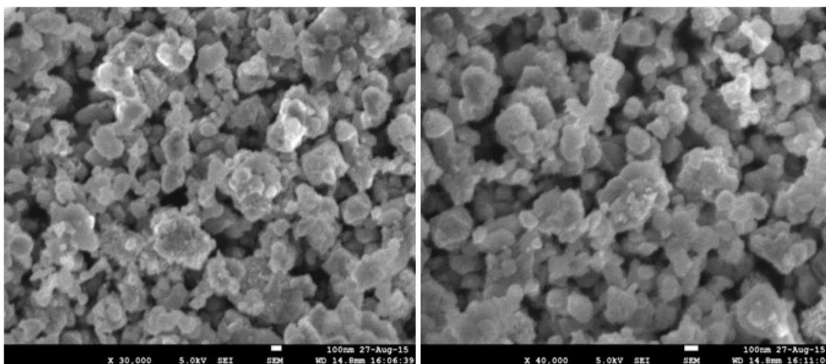
**Figure S1:** FE-SEM images of  $\text{Cu}(0)/\text{Fe}_3\text{O}_4$
