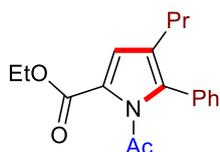
Colourless oil (43.0 mg, 72%);  $^1H$  NMR (500 MHz,  $CDCl_3$ )  $\delta$  7.36 – 7.28 (m, 3H), 7.22 – 7.17 (m, 2H), 6.82 (s, 1H), 4.23 (q,  $J = 7.1$  Hz, 2H), 2.25 – 2.19 (m, 2H), 2.18 (s, 3H), 1.43 (dd,  $J = 15.1, 7.5$  Hz, 2H), 1.28 (t,  $J = 7.1$  Hz, 3H), 0.78 (t,  $J = 7.4$  Hz, 3H);  $^{13}C$  NMR (100 MHz,  $CDCl_3$ )  $\delta$  173.5, 160.8, 135.4, 131.2, 130.1, 128.43, 128.37, 124.8, 123.2, 119.2, 60.7, 28.5, 27.4, 23.8, 14.3, 13.8.
