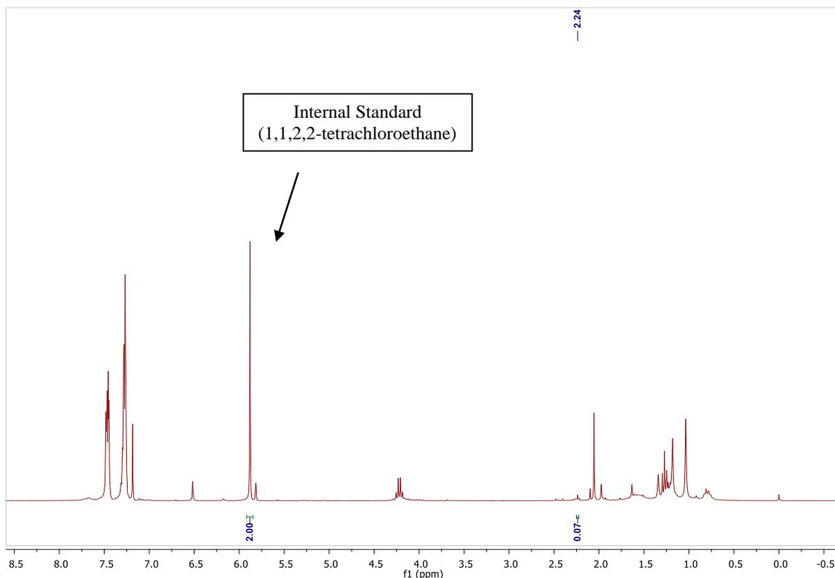
**Figure S2.** Crude <sup>1</sup>H NMR for reaction without oxidant.
