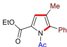
Colourless solid (47.0 mg, 87%);  $^1H$  NMR (400 MHz,  $CDCl_3$ )  $\delta$  7.37 – 7.29 (m, 3H), 7.24 – 7.19 (m, 2H), 6.79 (s, 1H), 4.23 (q,  $J = 7.1$  Hz, 2H), 2.19 (s, 3H), 1.91 (s, 3H), 1.27 (t,  $J = 7.1$  Hz, 3H);  $^{13}C$  NMR (100 MHz,  $CDCl_3$ )  $\delta$  173.6, 160.8, 135.5, 131.1, 129.9, 128.42, 128.37, 123.0, 120.3, 119.5, 60.7, 28.5, 14.3, 11.1.
