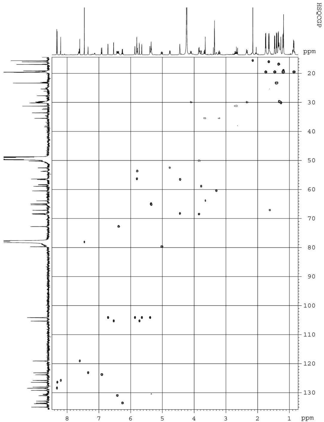
(E)HMBC spectrum of TSR-Ile1Met
