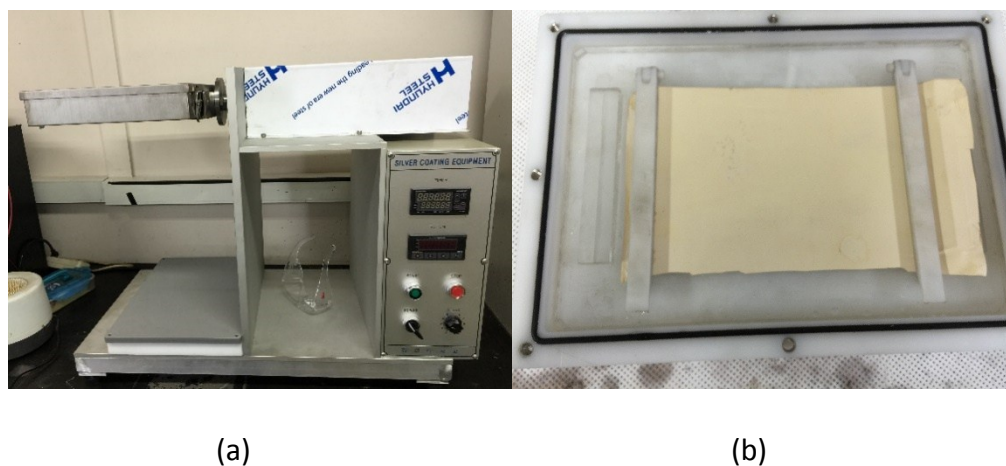
Fig. S1 (a) Silver plating equipment and (b) silver plating box; silver containing TPU nanofiber web (yellow web) is clipped inside the box. The silver plating box is made of a highly hydrophobic material, e.g., polyethylene.
