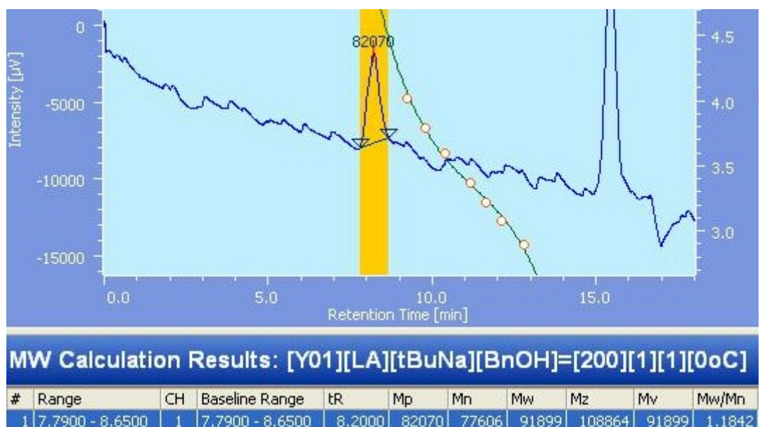
Figure S31. GPC result of PLA of entry 24
