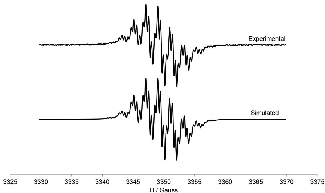
**Fig. S1.** EPR spectra of CN-BDPA (5) in  $\text{CH}_2\text{Cl}_2$  at 298 K: experimental (up) and simulated (down). EPR simulation data:  $g = 2.0024$ ;  $a(4\text{H}) = 1.928 \text{ G}$ ,  $a(4\text{H}) = 1.947 \text{ G}$ ,  $a(4\text{H}) = 0.492 \text{ G}$ ,  $a(4\text{H}) = 0.378 \text{ G}$ ;  $\Delta\text{Hpp} = 0.32 \text{ G}$ .
