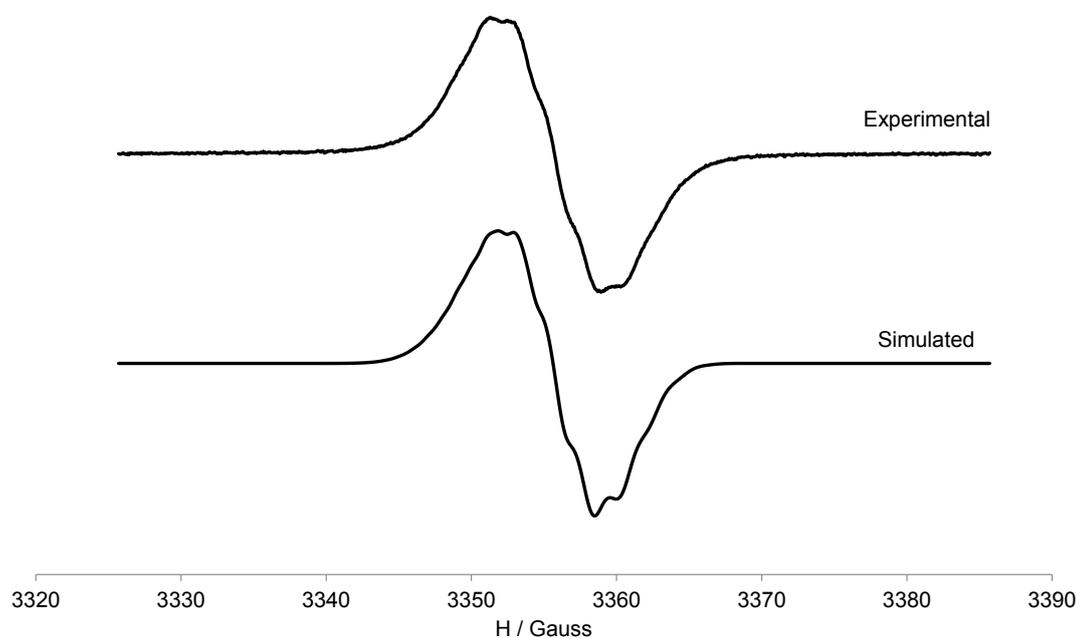
**Fig. S3.** Frozen solution EPR spectra of BAm-BDPA (7) in  $\text{CH}_2\text{Cl}_2$  at 120 K: experimental (up) and simulated (down). EPR simulation data:  $g_{xx} = 2.0010$ ;  $g_{yy} = 2.0026$ ;  $g_{zz} = 2.0048$ ;  $a(8\text{H}_a)$ :  $a_{xx} = 1.85$  G,  $a_{yy} = 1.85$  G,  $a_{zz} = 2.00$  G;  $a(8\text{H}_b)$ :  $a_{xx} = 0.45$  G,  $a_{yy} = 0.45$  G,  $a_{zz} = 0.90$  G;  $\Delta\text{Hpp} = 1.0$  G.
