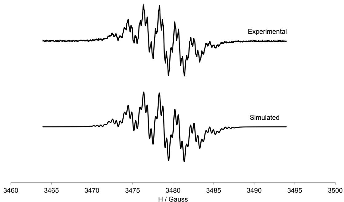
**Fig. S2.** EPR spectra of BAm-BDPA (**7**) in  $\text{CH}_2\text{Cl}_2$  at 298 K: experimental (up) and simulated (down). EPR simulation data:  $g = 2.0023$ ;  $a(4\text{H}) = 2.002$  G,  $a(4\text{H}) = 1.835$  G,  $a(4\text{H}) = 0.465$  G,  $a(4\text{H}) = 0.394$  G;  $\Delta H_{\text{pp}} = 0.25$  G.
