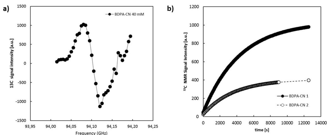
**Fig. S4** a)  $^{13}\text{C}$  microwave spectrum of 100  $\mu\text{l}$  of a 1:1 (v/v)  $[1-^{13}\text{C}]$ pyruvic acid:sulfolane doped with 40 mM CN-BDPA **5** at 3.35 T and 1.4 K. b)  $^{13}\text{C}$  polarization build-up curves of 30  $\mu\text{l}$  1:1
