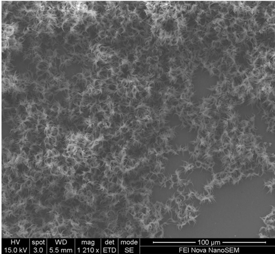
**Fig. S5** SEM of TTPEcNDI in the THF/water ( $f_w = 80\%$ ).
