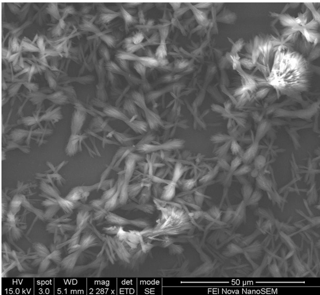
**Fig. S3** SEM of TTPEcNDI in the CHCl<sub>3</sub>/MeOH ( $f_m = 80\%$ ).
