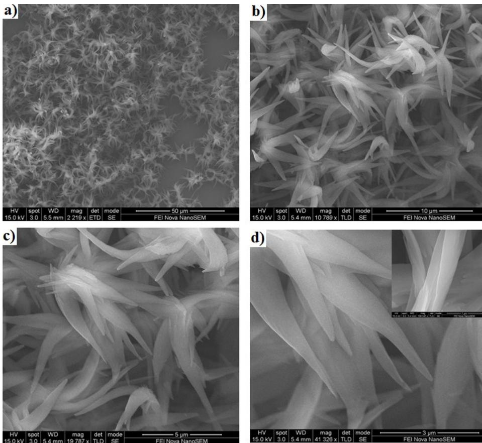
**Fig. S6** SEM of TTPEcNDI in the THF/water ( $f_w = 70\%$ ).
