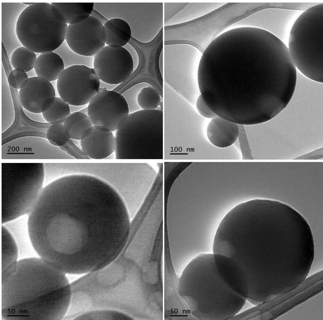
**Fig. S8** TEM images of **TTPEcNDI** in the  $\text{CHCl}_3/\text{hexane}$  ( $f_h = 90\%$ ).
