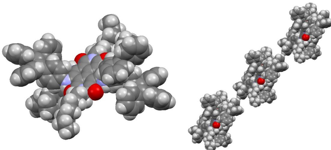
**Figure S11.** Space filling model of TTPEcNDI 1
