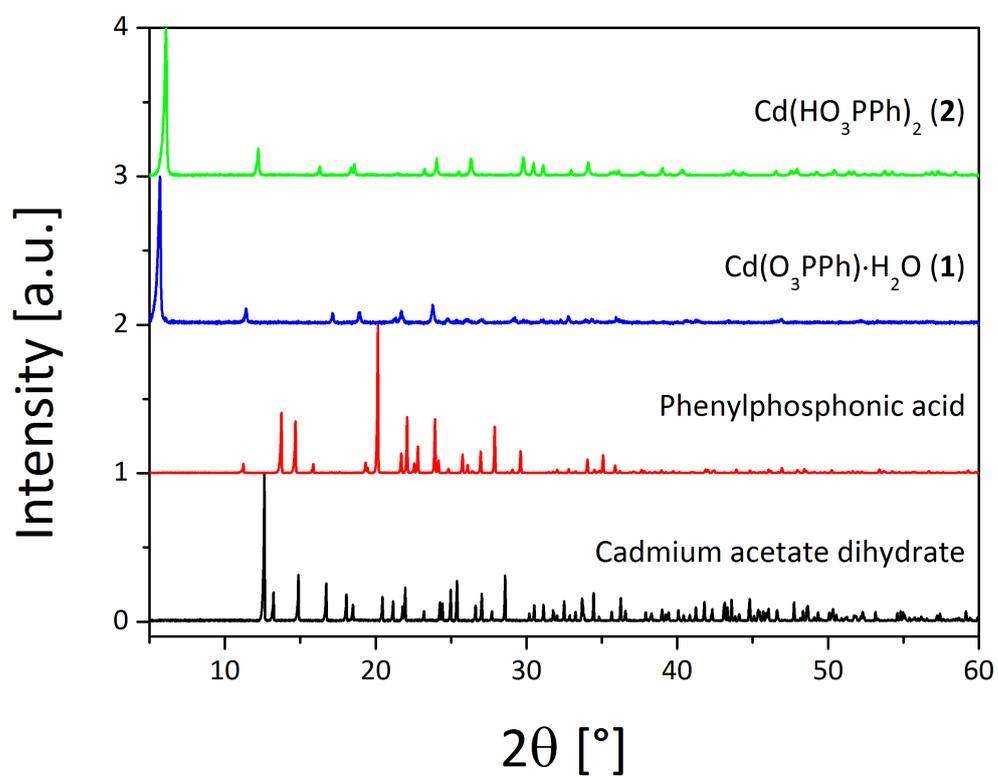
Figure S1: Comparison of the measured PXRD patterns of (1) (blue) and (2) (green) with the measured PXRD patterns of the starting materials cadmium acetate dihydrate (black) and phenylphosphonic acid (red).
