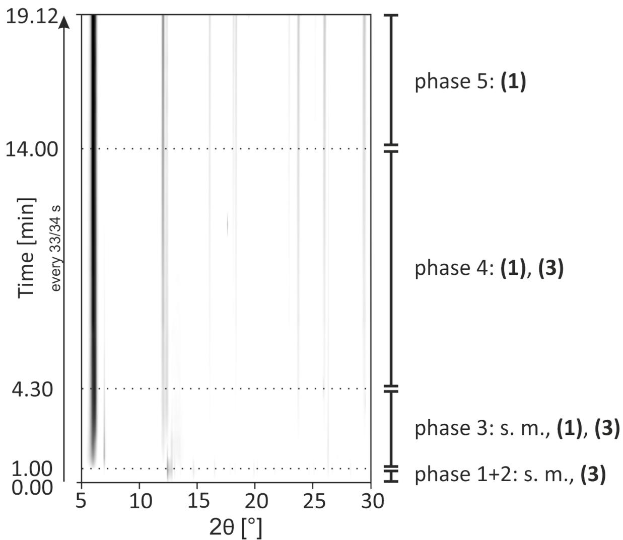
Figure S4: 2D plot of synchrotron XRD data for the synthesis of (1).
