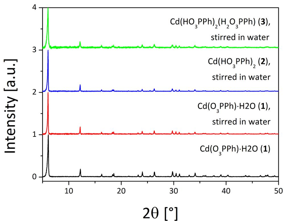
Figure S8: XRD patterns after slurry experiments to obtain the relative stability of the compounds (1)-(3). Each compound (250 mg) was stirred for 24 h in water (25 ml) under ambient conditions. The solid phase was gained by filtration and analyzed by powder X-ray diffraction (PXRD). Compound 1 was obtained as single product in all three cases.
