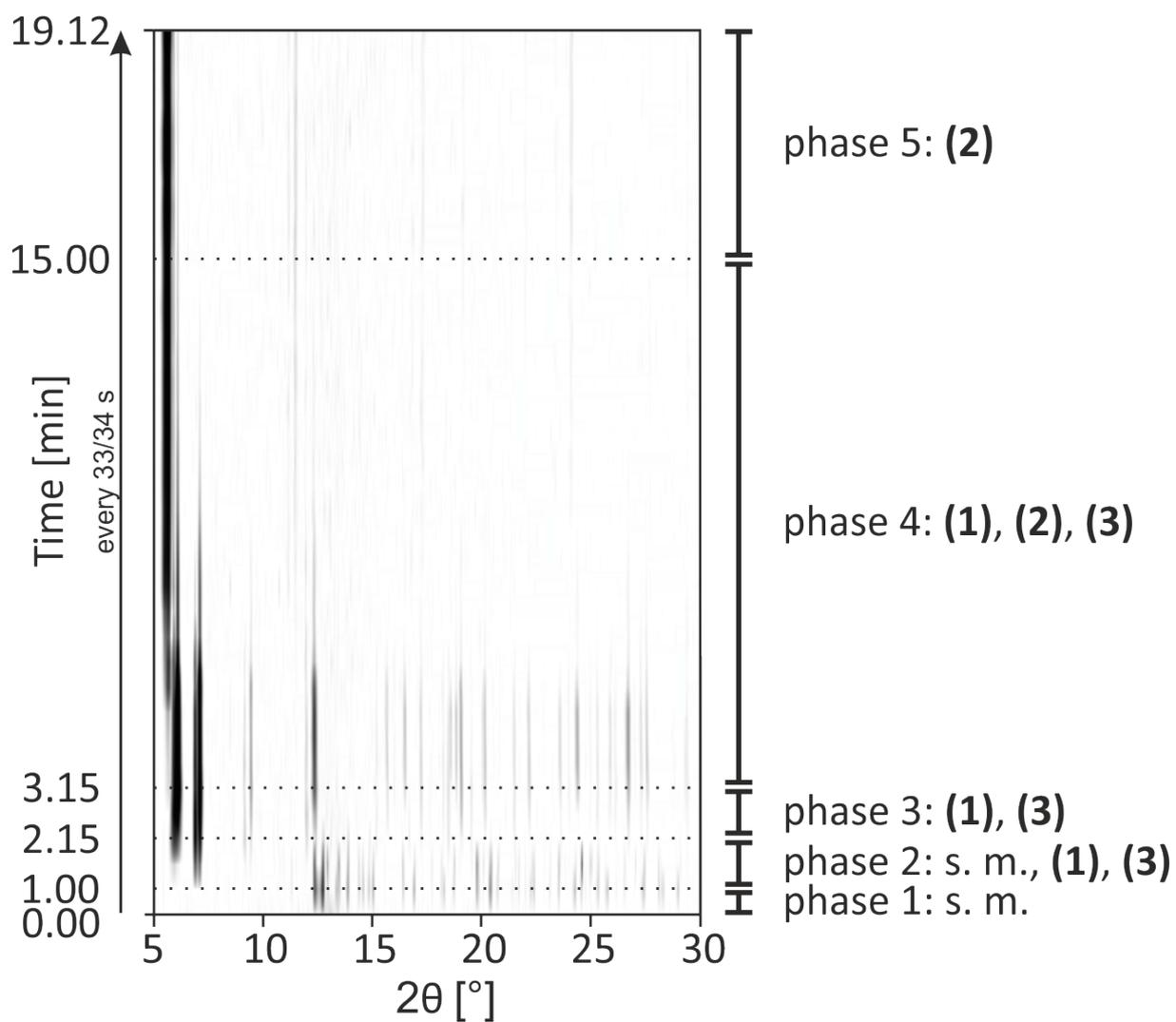
Figure S5: 2D plot of synchrotron XRD data for the synthesis of **(1)**.
