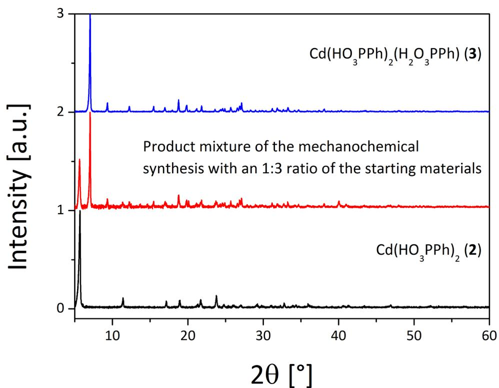
Figure S3: Comparison of the measured PXRD pattern of the product mixture of the mechanochemical synthesis of cadmium acetate with phenylphosphonic acid in a 1:3 ratio (red) with the measured PXRD patterns of (2) (blue) and (3) (black).
