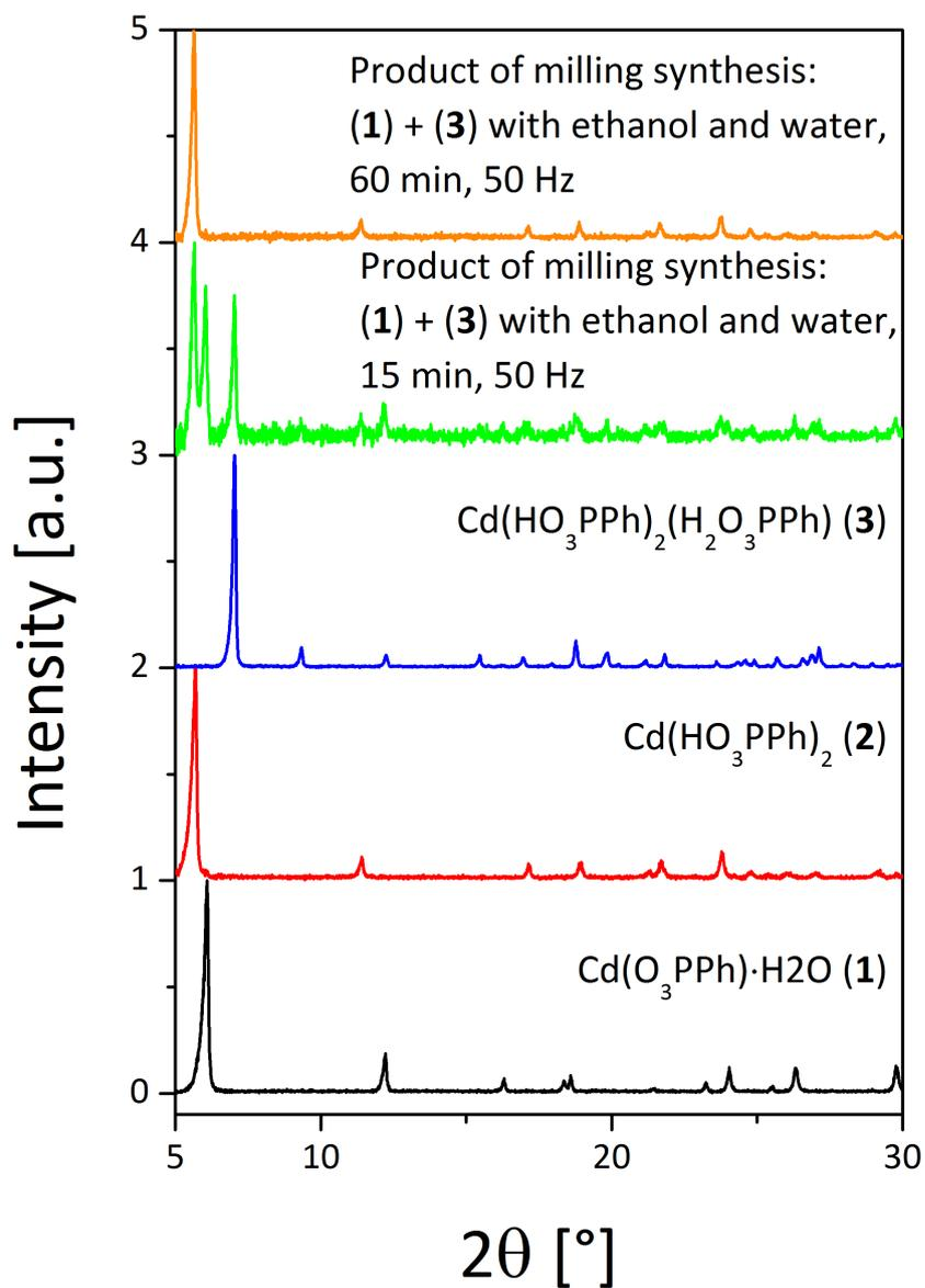
Figure S7: XRD patterns of the products of the syntheses milling compound (**1**) and (**3**) together for 15 min (green) or 60 min (orange) at 50 Hz. Reactions were carried out by milling (**1**) and (**3**) in a molar ratio of 1:1 and a total load of 1 g together with acetic acid (200 L) and water (50 L) as liquid assistants.
