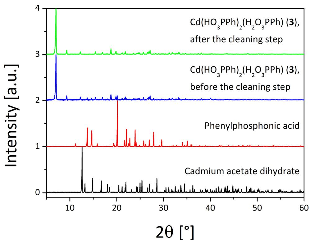
Figure S2: Comparison of the measured PXRD patterns of (**3**) after the mechanochemical synthesis, before the cleaning step (blue) and (**3**) after stirring in diethyl ether (green) with the measured PXRD patterns of the starting materials cadmium acetate dihydrate (black) and phenylphosphonic acid (red).
