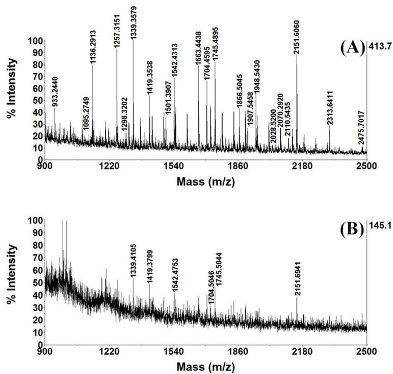
**Fig. S9.** MALDI mass spectra of N-glycans enriched from ovalbumin digests with different concentrations (A) 5 ng/μL; (B) 2 ng/μL, using Mag-NHCs.
