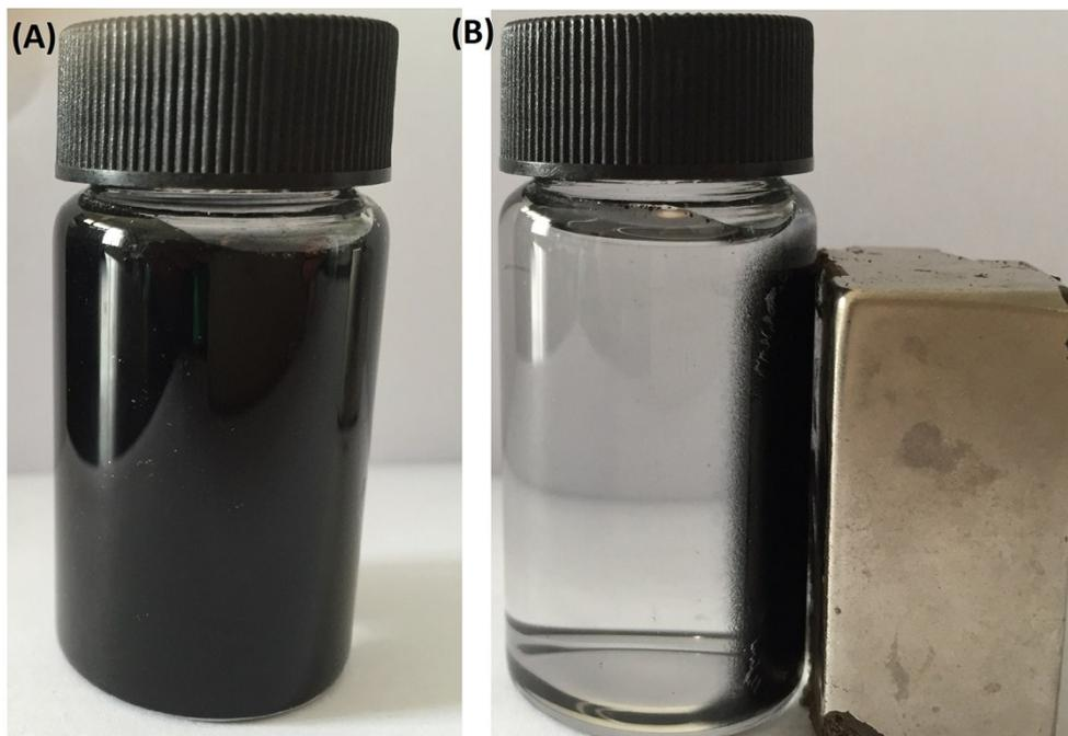
**Fig. S4.** Mag-NHCs dispersed in water (A) and magnetically separated (B).
