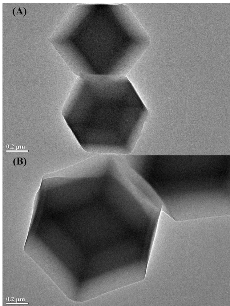
**Fig. S2.** TEM images of (A) ZIF-8 crystals; (B) ZIF-8@ZIF-67 crystals.
