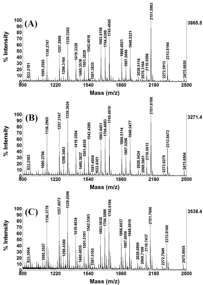
**Fig. S8.** MALDI mass spectra of N-glycans enriched from ovalbumin digests (10 μg) by Mag-NHCs (50 μL, 10 mg/mL, in water). (A) first application of the materials; (B) second application of the materials; (C) third application of the materials.
