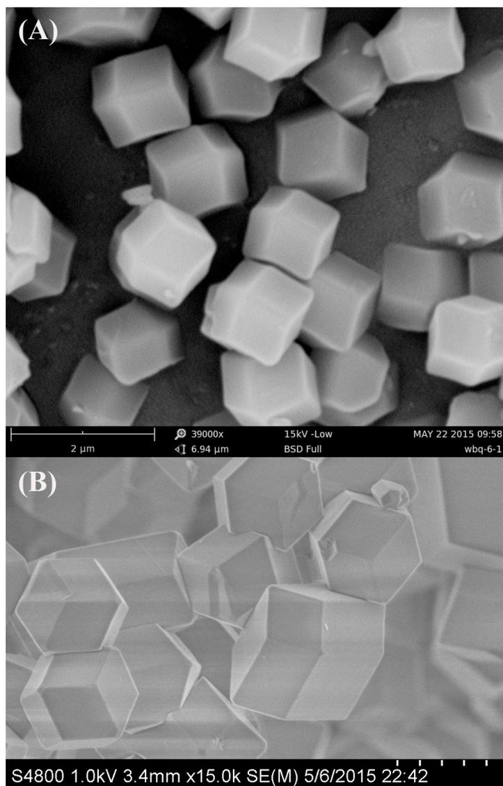
**Fig. S1.** SEM images of (A) ZIF-8 crystals; (B) ZIF-8@ZIF-67 crystals.
