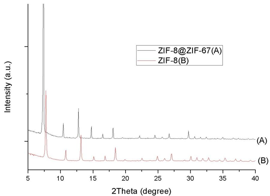
**Fig. S3.** Wide-angle XRD pattern of (A) ZIF-8@ZIF-67 crystals; (B) ZIF-8 crystals.
