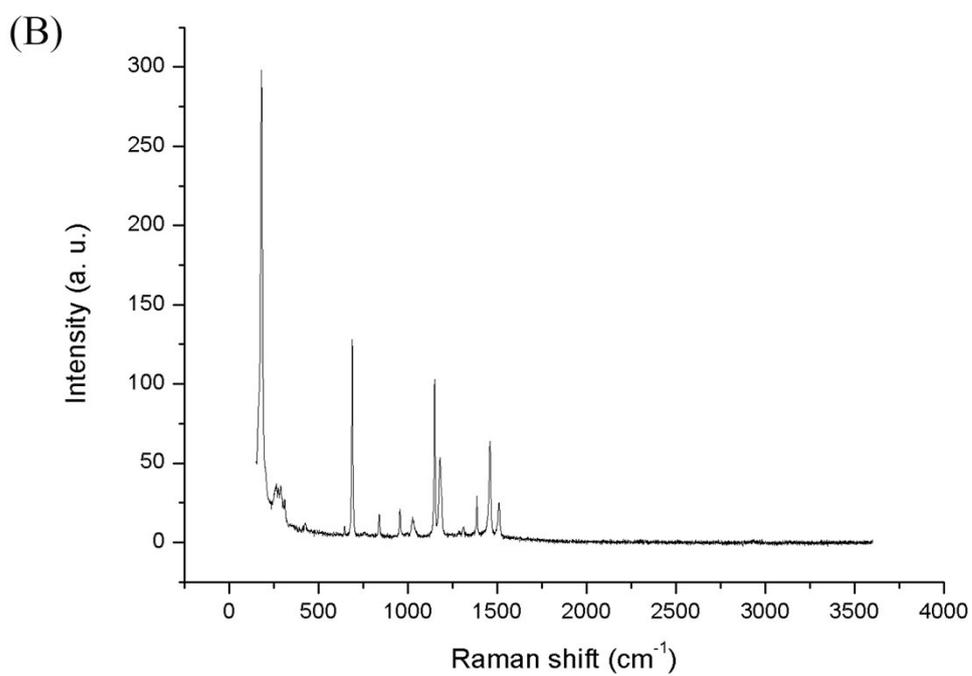
**Fig. S6.** Raman spectrum of (A) ZIF-8 crystals; and (B) ZIF-8@ZIF-67 crystals.
