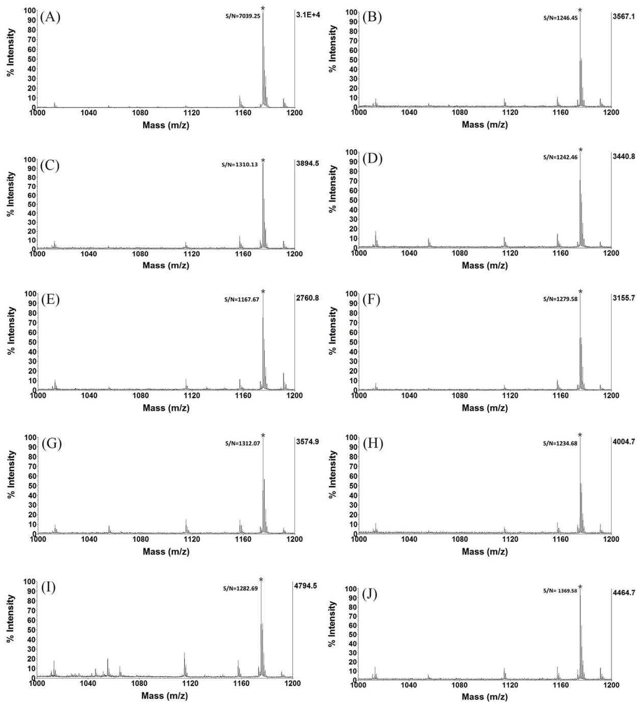
**Fig. S10.** MALDI mass spectra of (A) 500 ng of maltoheptaose and (B-J) the elution (5 $\mu$ L, 1 $\mu$ L was spotted on the MALDI plate) after enrichment with Mag-NHCs.
