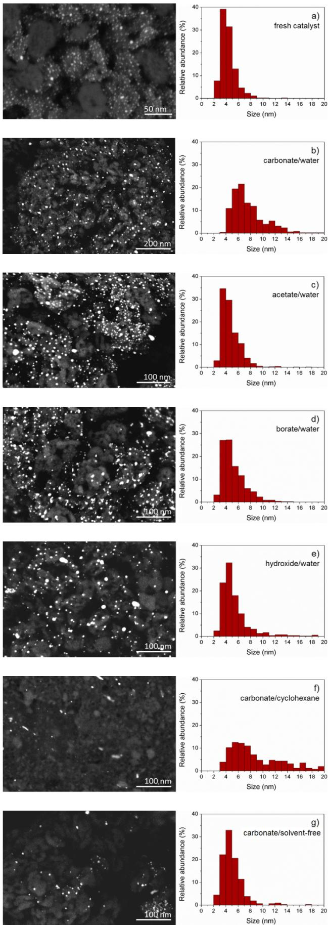
**Figure S1.** STEM images before and after being exposed to different reaction conditions. a) fresh catalyst, b)  $\text{K}_2\text{CO}_3/\text{water}$ , c)  $\text{Na}(\text{CH}_3\text{COO})/\text{water}$ , d)  $\text{Na}_2\text{B}_4\text{O}_7/\text{water}$ , e)  $\text{NaOH}/\text{water}$ , f)  $\text{K}_2\text{CO}_3/\text{cyclohexane}$  and g)  $\text{K}_2\text{CO}_3/\text{solvent-free}$ .
