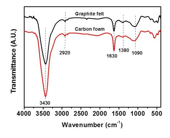
3 Fig. S1 FT-IR spectra of the graphite felt and the as-synthesized carbon foam.
