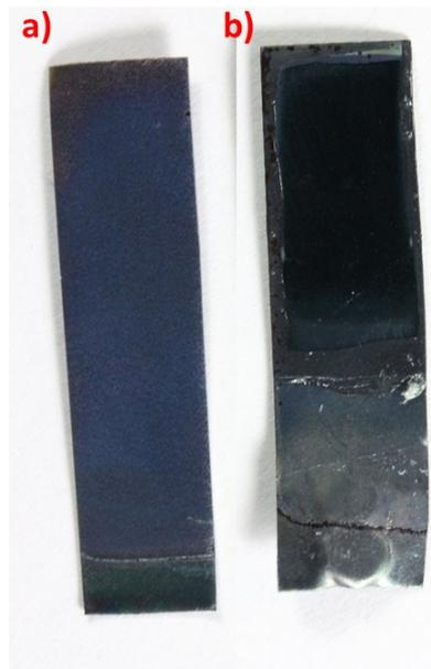
**Fig. S3** Photography of a) H-TiO<sub>2</sub>NTs and b) H-TiO<sub>2</sub>NTs/pEDOT:PSS sample.
