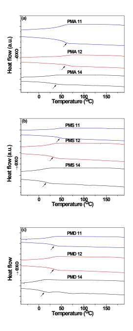
Figure S1. DSC curves of different polyesters (a) PMA (b) PMS (c) PMD showing the cooling and heating curves. The arrows indicate the transition indicating the glass transition temperature.
