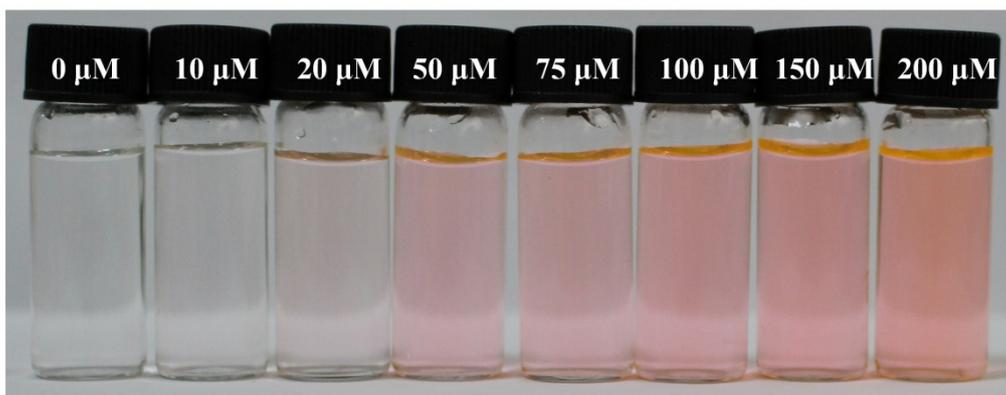
**Fig. S9** The photographs of the R6G-CD nanosensor in the absence of Fe<sup>3+</sup> and upon addition of Fe<sup>3+</sup> in aqueous solution.
