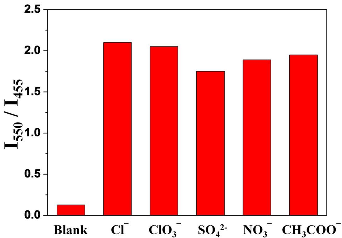
**Fig. S13** Fluorescence intensity ratio ( $I_{550}/I_{455}$ ) of the R6G-CD nanosensor (0.02 mg/mL) in the presence of 200  $\mu$ M various Fe<sup>3+</sup> salts (Cl<sup>-</sup>, ClO<sub>3</sub><sup>-</sup>, SO<sub>4</sub><sup>2-</sup>, NO<sub>3</sub><sup>-</sup>, CH<sub>3</sub>COO<sup>-</sup>), respectively.
