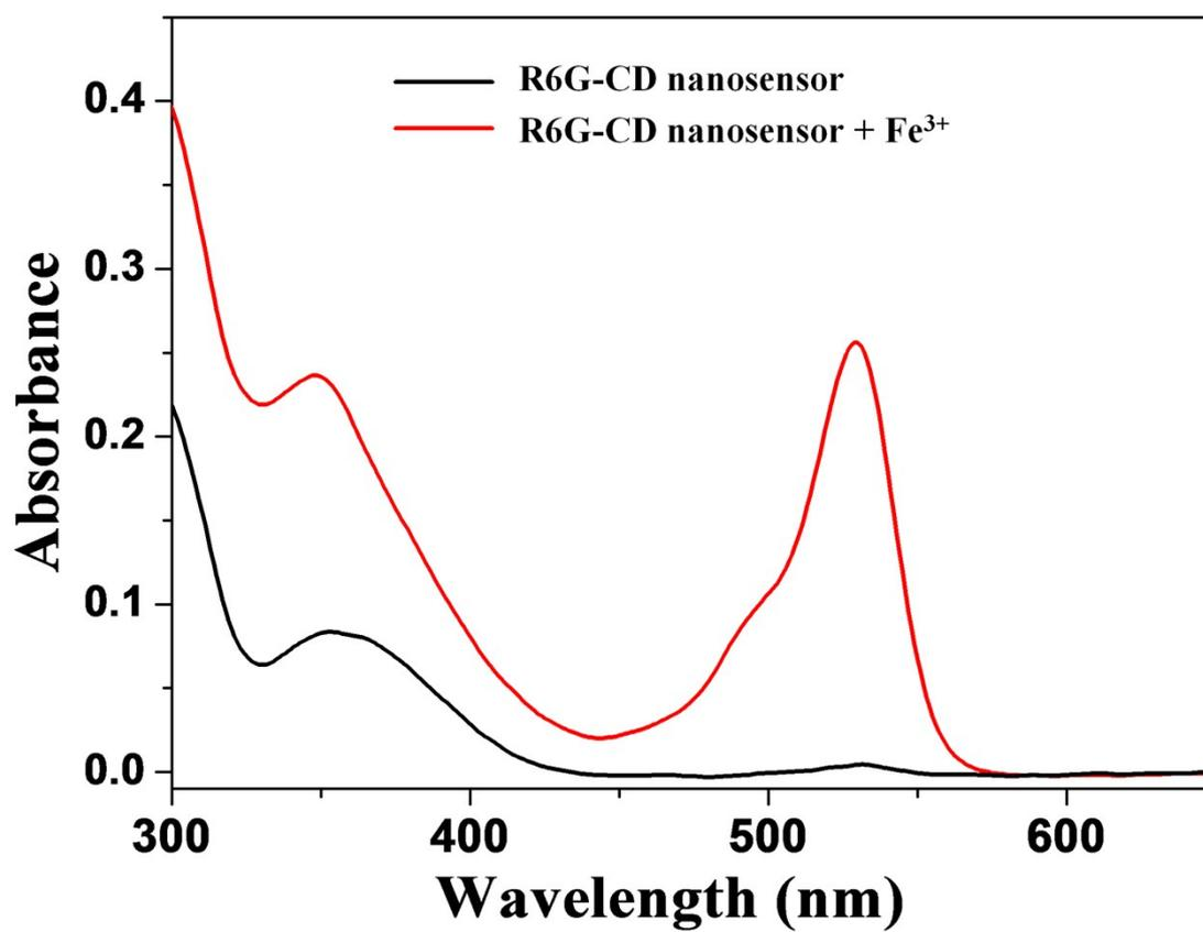
**Fig. S8** Absorption spectra of R6G-CD nanosensor (0.02 mg/mL) in aqueous solution before and after addition of Fe<sup>3+</sup>.
