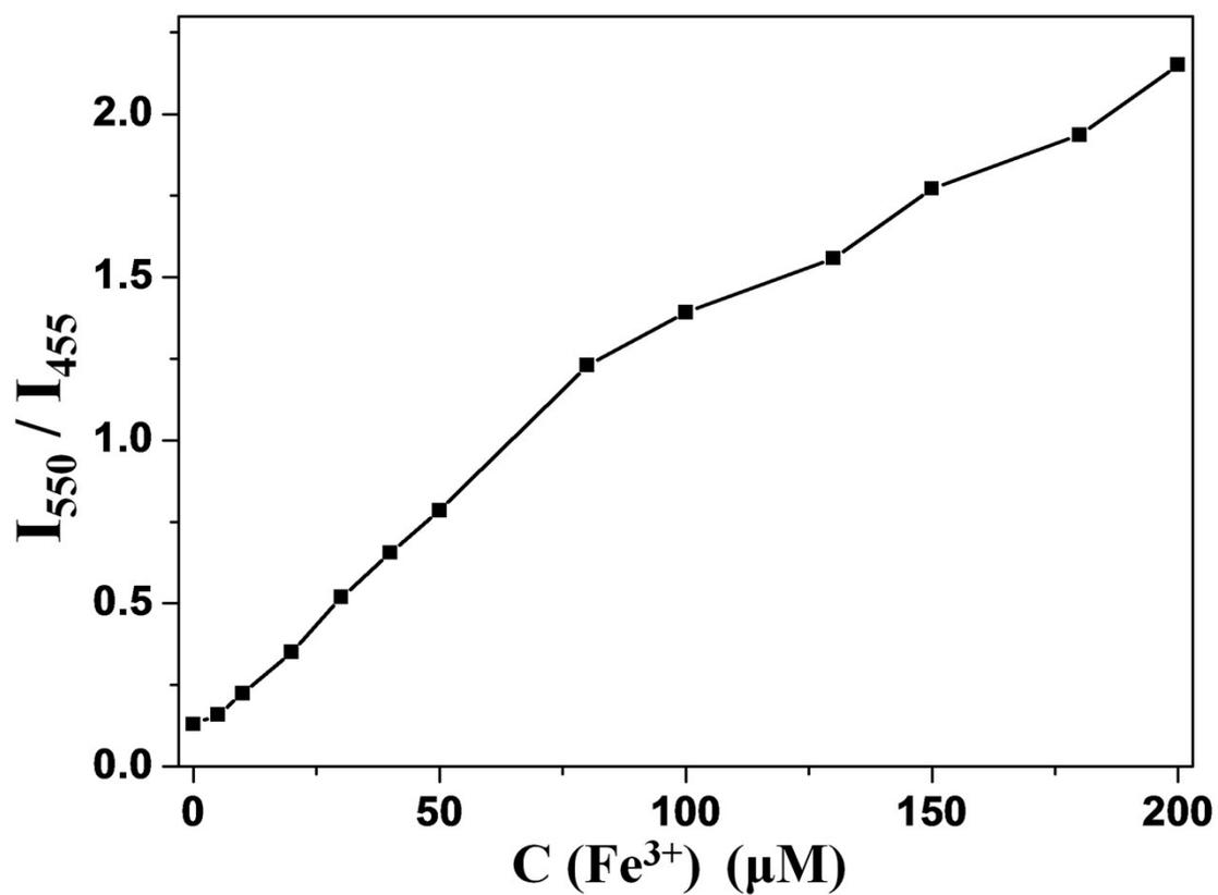
**Fig. S10** Fluorescent intensity ratio ( $I_{550}/I_{455}$ ) of the R6G-CD nanosensor (0.02 mg/mL) in the presence of different amounts of  $\text{Fe}^{3+}$  in aqueous solution ( $\lambda_{\text{ex}} = 360$  nm).
