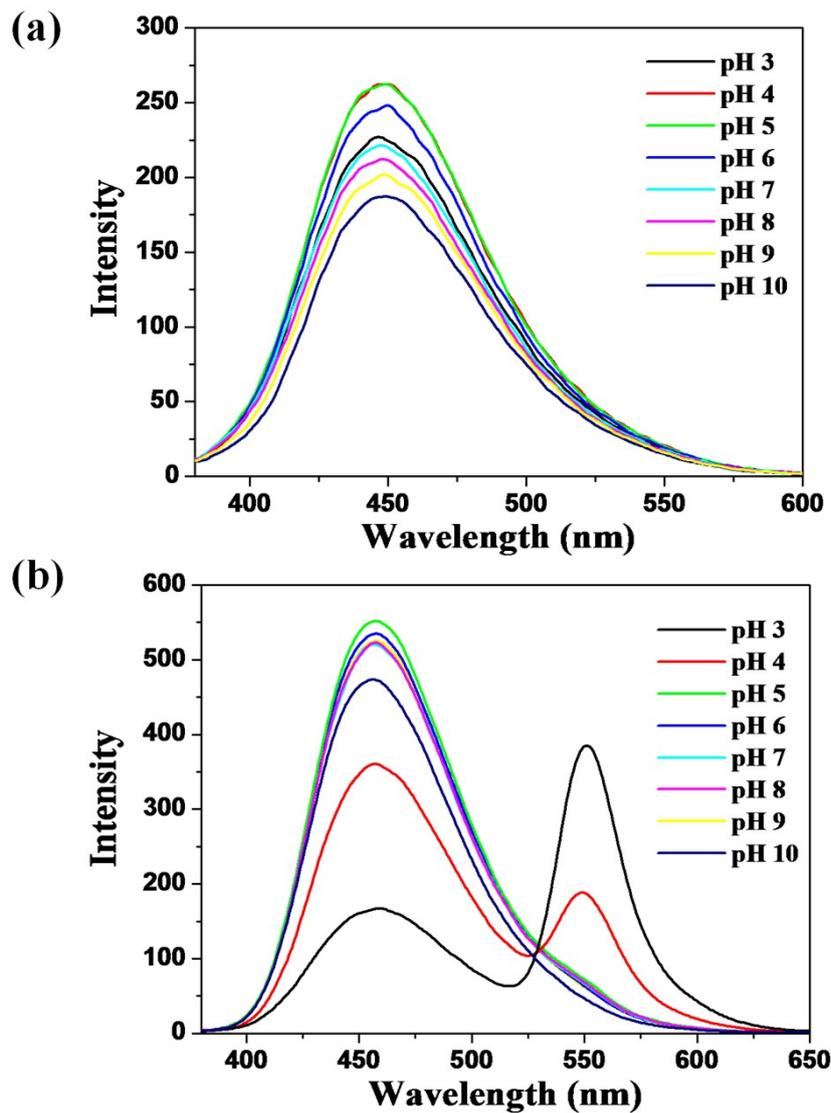
**Fig. S7** The fluorescence spectra of (a) the CDs (0.01 mg /mL) and (b) the R6G-CD nanosensor (0.02 mg /mL) in pH 3-10 Britton–Robinson buffer solution (40 mM) ( $\lambda_{\text{ex}} = 360$  nm).
