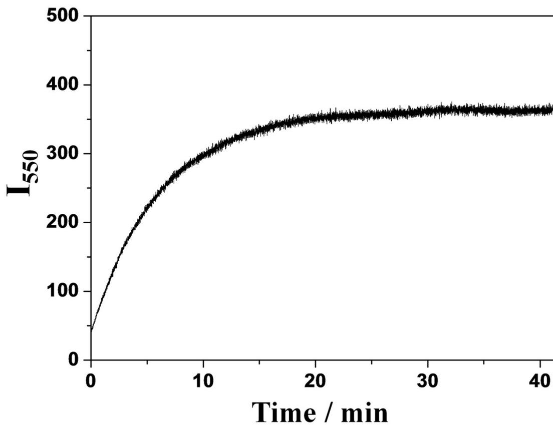
**Fig. S11** Fluorescence intensity ( $I_{550}$ ) of the R6G-CD nanosensor (0.02 mg /mL) upon addition of 200  $\mu\text{M}$   $\text{Fe}^{3+}$  in water.
