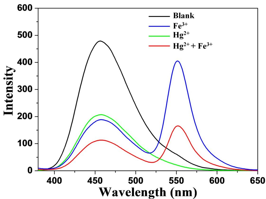
**Fig. S12** The fluorescence spectra of the R6G-CD nanosensor (0.02 mg/mL) (a) in the absence or in the presence of 200  $\mu$ M (b) Fe<sup>3+</sup>, (c) Hg<sup>2+</sup> and (d) Fe<sup>3+</sup> + Hg<sup>2+</sup> in aqueous solution ( $\lambda_{\text{ex}} = 360$  nm).
