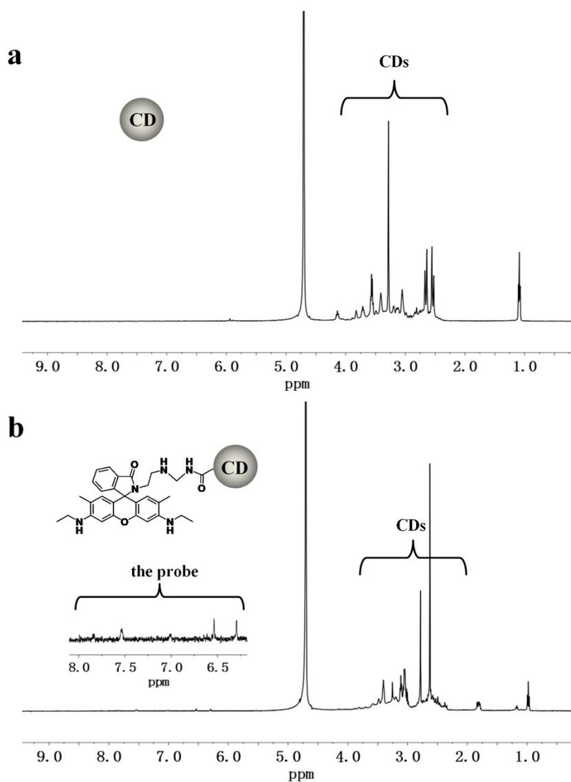
**Fig. S5**  $^1\text{H}$  NMR spectra (in  $\text{D}_2\text{O}$ ) of (a) the plain CDs and (b) the R6G-CD nanosensor.
