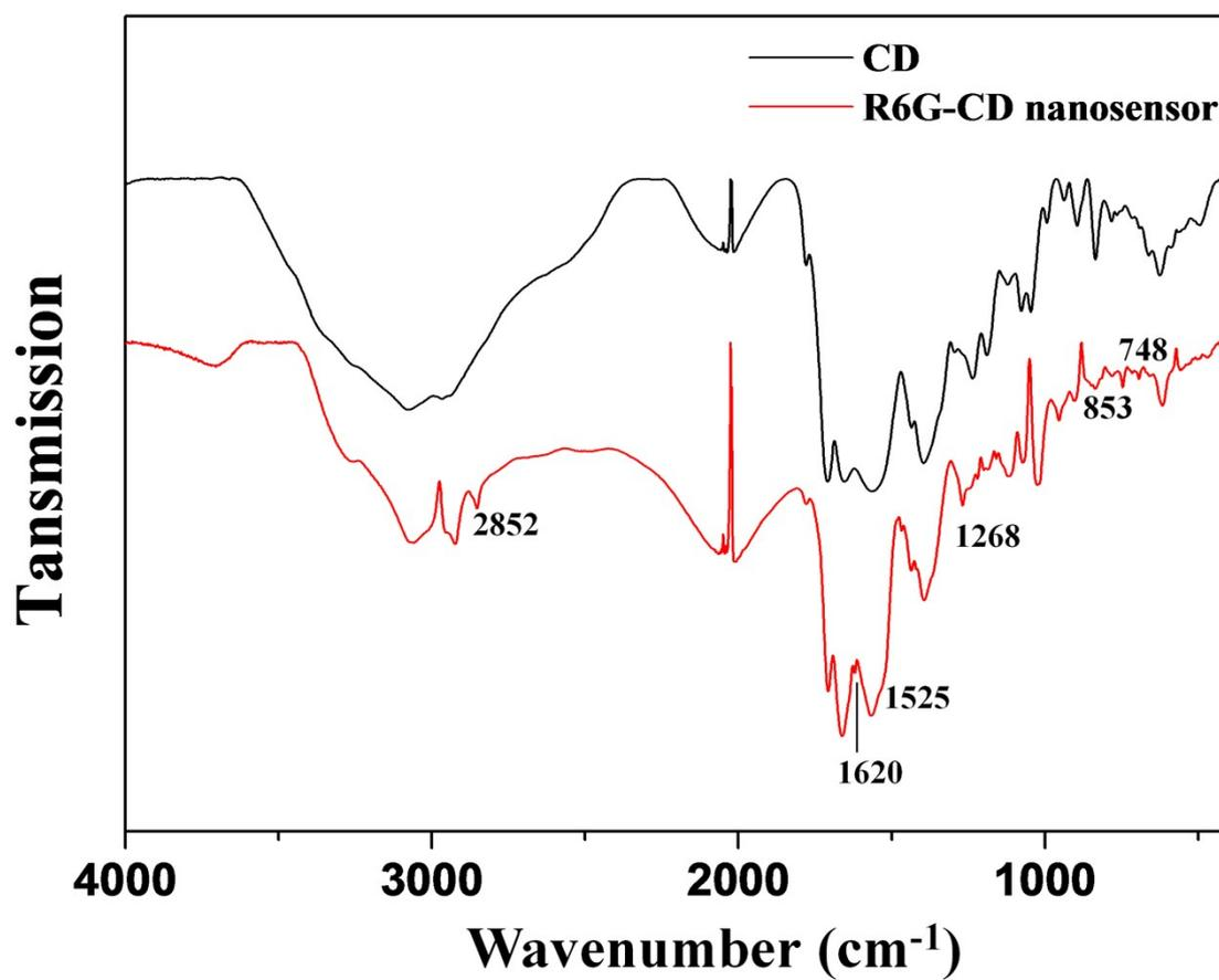
Fig. S6 FTIR spectra of the plain CDs (black) and the R6G-CD nanosensor (red).
