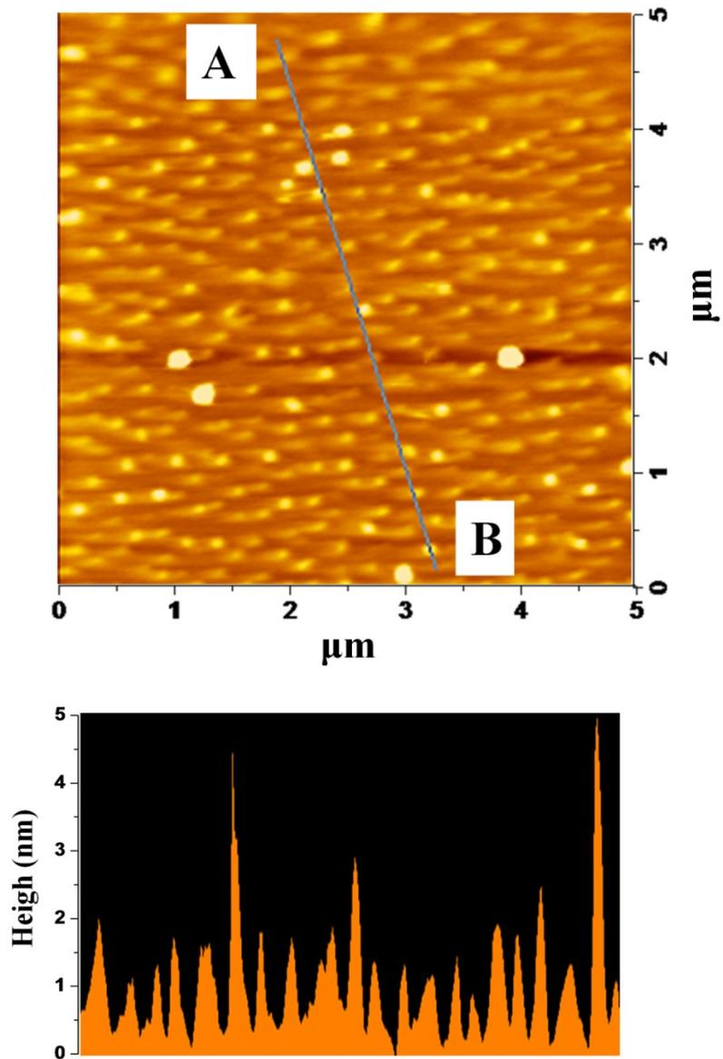
**Fig. S1** AFM topography image of CDs with height profile along line AB in the image.
