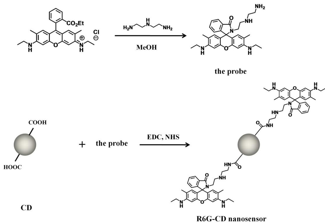
**Scheme S1** Synthesis route for the R6G-CD nanosensor.
