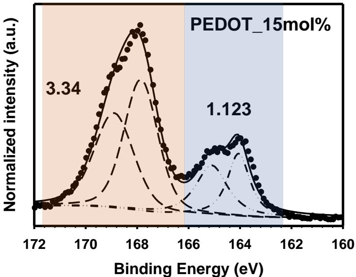
Figure 4. S2p spectra of pristine PEDOT:PSS and PEDOT:P(SS-co-PEGMA) thin films and deconvolution graphs of S2p spectra, without DMSO post-treatment
