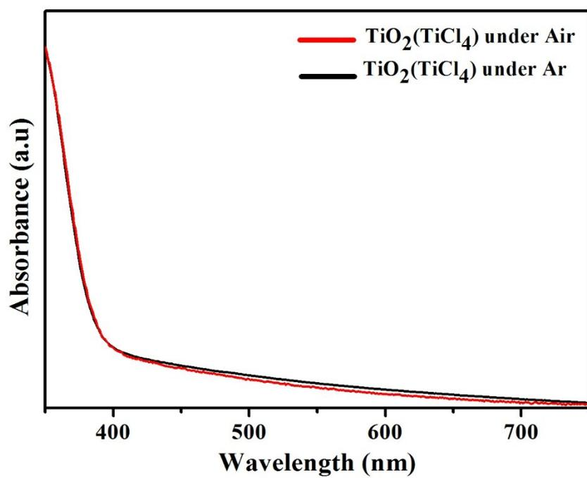
**Fig. S4** UV-vis DRS of annealed TiO<sub>2</sub> under Air and Ar atmosphere.
