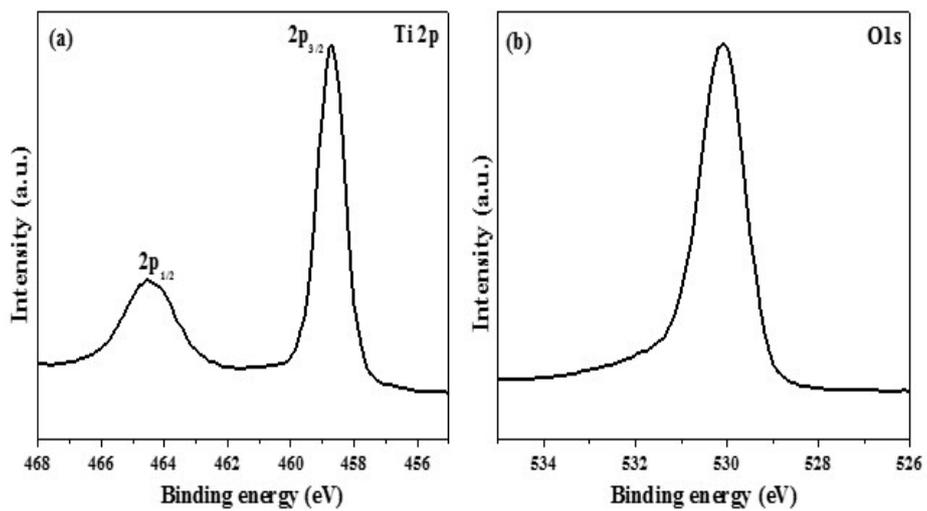
**Fig. S5** X-ray photoelectron spectroscopy (XPS) of as synthesized TiO<sub>2</sub> showing the regions of (a) Ti 2p, and (b) O1s.
