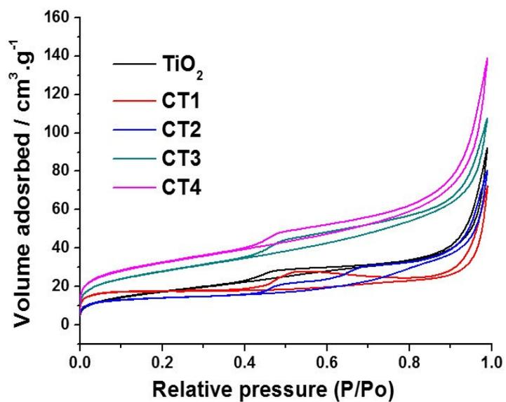
**Fig. S7** Nitrogen physisorption isotherms for BET surface area measurement for pure TiO<sub>2</sub> and hybrid mesoporous CZTS-TiO<sub>2</sub> samples (CT1, CT2, CT3 and CT4 stands for 1.9, 3.8, 5.7 and 7.6 mg of CZTS in TiCl<sub>4</sub> respectively).
