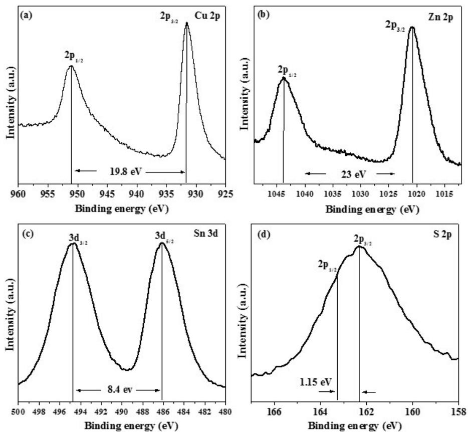
**Fig. S6** X-ray photoelectron spectroscopy (XPS) of as-prepared CZTS nanoparticles showing the regions of (a) Cu 2p, (b) Zn 2p, (c) Sn 3d, and (d) S 2p.
