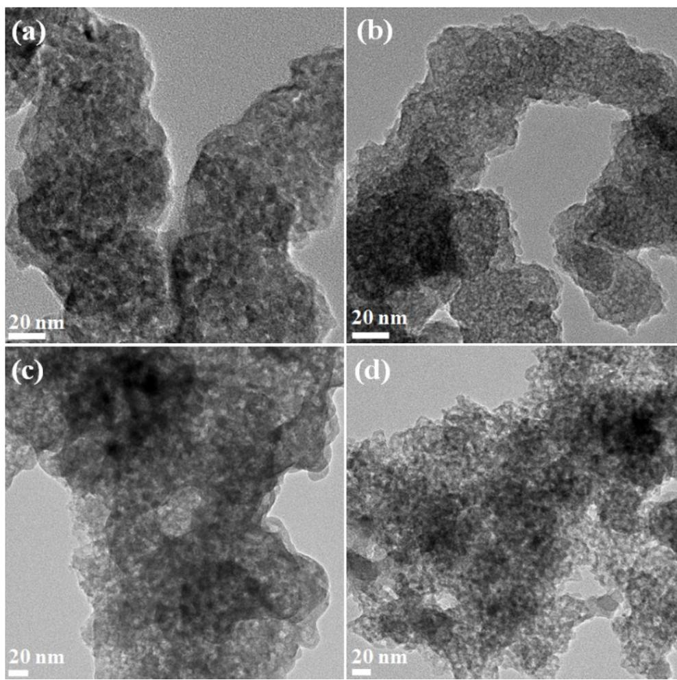
**Fig. S2** TEM images of hybrid mesoporous CZTS-TiO<sub>2</sub> samples: (a) CT1, (b) CT2, (c) CT3 and (d) CT4. (CT1, CT2, CT3 and CT4 stands for 1.9 mg, 3.8 mg, 5.7 mg and 7.6 mg of CZTS for 0.1 ml of TiCl<sub>4</sub> respectively)
