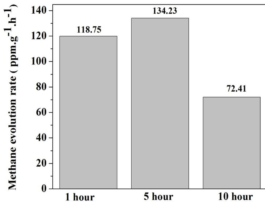
**Fig. S8** Stability test employing sample CT4, synthesized from 7.6 mg CZTS in 0.1 ml TiCl<sub>4</sub>, for CO<sub>2</sub> photoreduction under continuous simulated solar light illumination for 5 h and 10 h.
