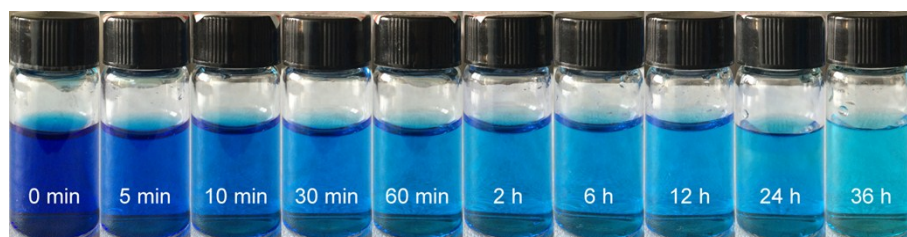
Figure S4. Digital pictures for the MB solution ( 100 \text{ mg L}^{-1} , 20\text{mL} ) and those after treatment with \text{Mg}(\text{OH})_2/\text{GO} composite ( 20\text{mg} ) at different time.
