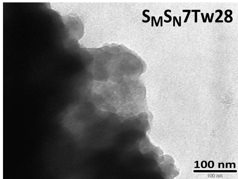
**Fig. S2** TEM images of hybrid mixed-structure silicas using Tween®80,  $S_M S_N Tw28$ .
