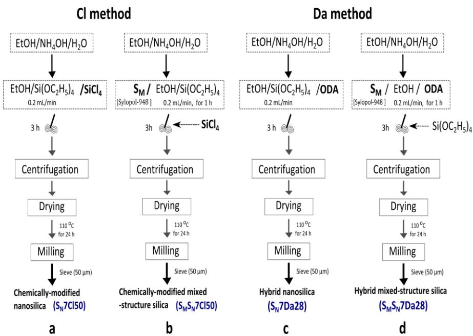
**Scheme S1.** Steps employed for the synthesis of  $S_N7Cl50$  (a),  $S_M S_N 7Cl50$  (b),  $S_N7Da28$  (c), and  $S_M S_N 7Da28$  (d) using a TEOS/ethanol molar ratio of 0.07, a TEOS/SiCl<sub>4</sub> molar ratio of 5.0, and 0.0028 mol of ODA.
