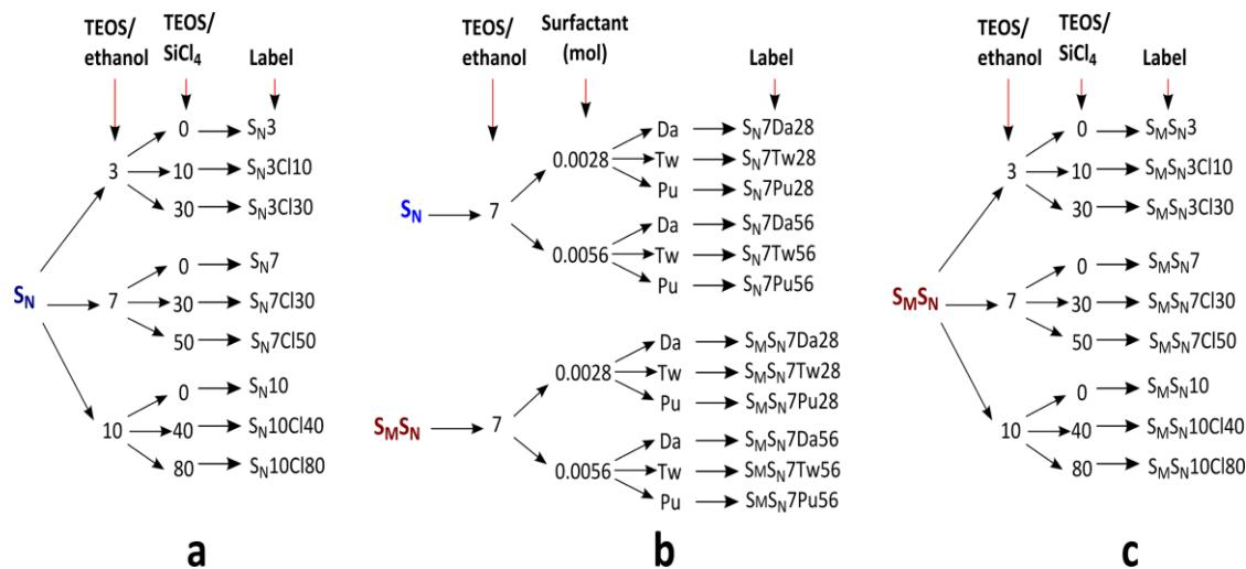
**Scheme S2.** The experimental approach for the syntheses of silica samples.<sup>5</sup>
