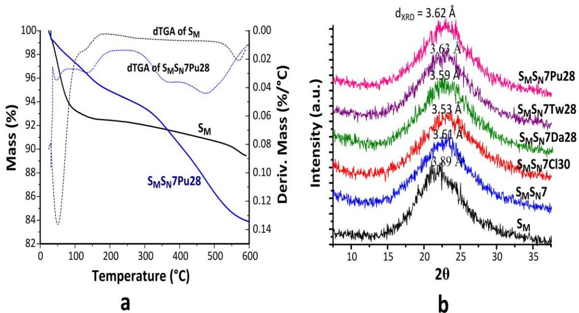
**Fig. S1** (a) TGA and DTGA curves of  $S_M$  (black) and  $S_M S_N 7Pu28$  (blue); heating  $20 \text{ \textdegree C}.\text{min}^{-1}$ . (b) X-Ray diffraction spectra of  $S_M$  compared with  $S_M S_N Cl30$ ,  $S_M S_N 7Da28$ ,  $S_M S_N 7Tw28$ , and  $S_M S_N 7Pu28$ .
