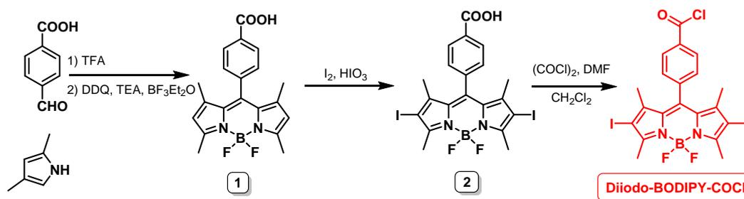
**Scheme S1.** The synthetic route of Diiodo-BODIPY-COCl.
