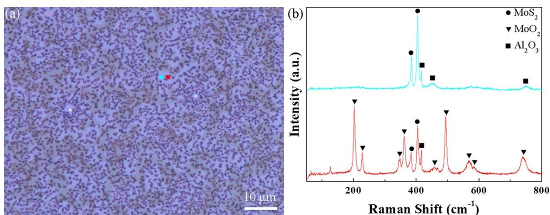
**Figure S4.** (a) Larger version of the image taken at  $D_{\text{dist}} = 15.0$  cm. (b) Raman spectra acquired from different regions highlighted in (a). These results illustrate that the initially formed monolayer MoS<sub>2</sub> grows around MoO<sub>2</sub> domains.
