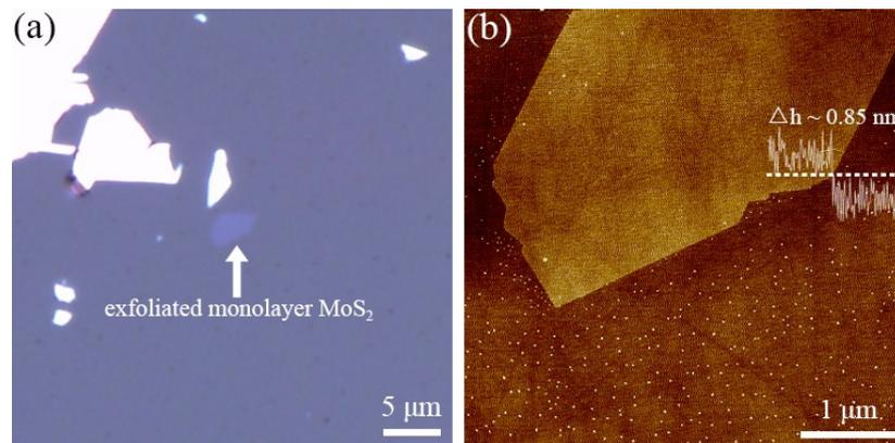
**Figure S2.** (a) Optical microscope image and (b) atomic force microscope image of the exfoliated monolayer MoS<sub>2</sub> sample. Section-view along the white dash line shows that the sample thickness is about 0.85 nm, which confirms the monolayer nature of the exfoliated MoS<sub>2</sub> sample.
