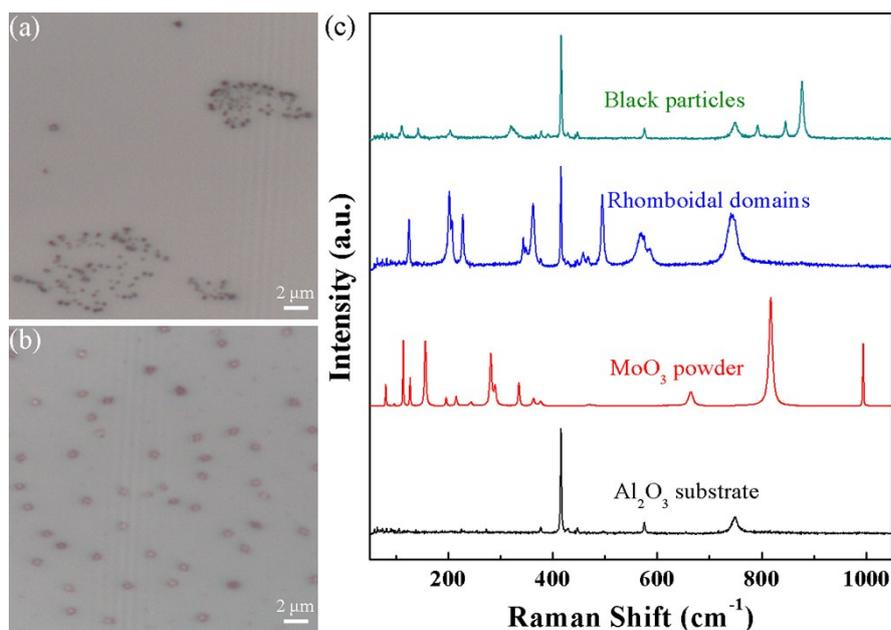
**Figure S3.** Optical microscope images of (a) the small black particles and (b) rhomboidal shaped domains. (c) Raman spectra of the small black particles, rhomboidal shaped domains, MoO<sub>3</sub> powder, and the bare sapphire substrate, respectively.
