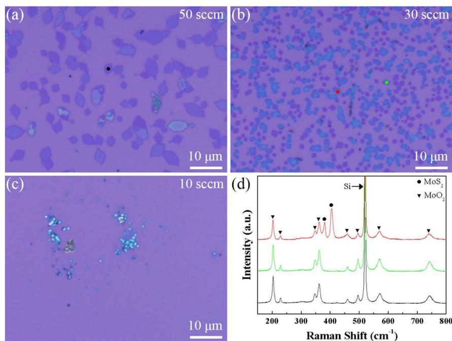
**Figure S6.** (a-c) Optical microscope images of the products synthesized with different Ar flow rate of 50, 30, and 10 sccm, respectively, SiO<sub>2</sub>/Si substrates are located at the center of furnace. (d) Raman spectra acquired from different samples and different regions highlighted in (a) and (b).
