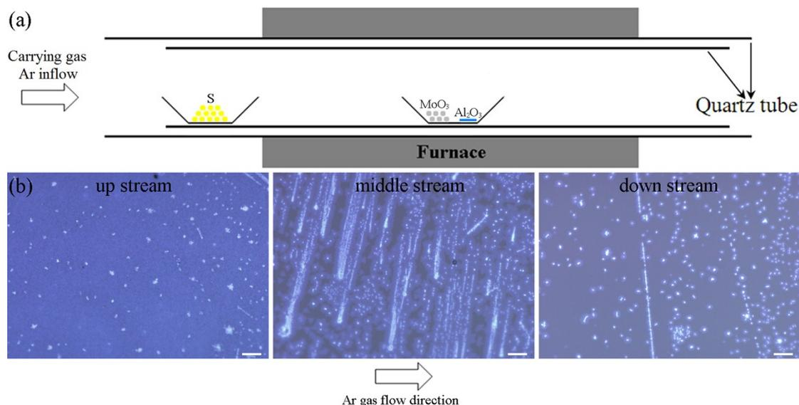
**Figure S1.** (a) Schematic illustration for MoS<sub>2</sub> growth on Al<sub>2</sub>O<sub>3</sub> (0001) substrate with sulfur powder placed upstream. (b) Optical microscope images of synthesized MoS<sub>2</sub> on sapphire taken along the Ar gas flow direction. The scale bars are 10  $\mu\text{m}$ .
