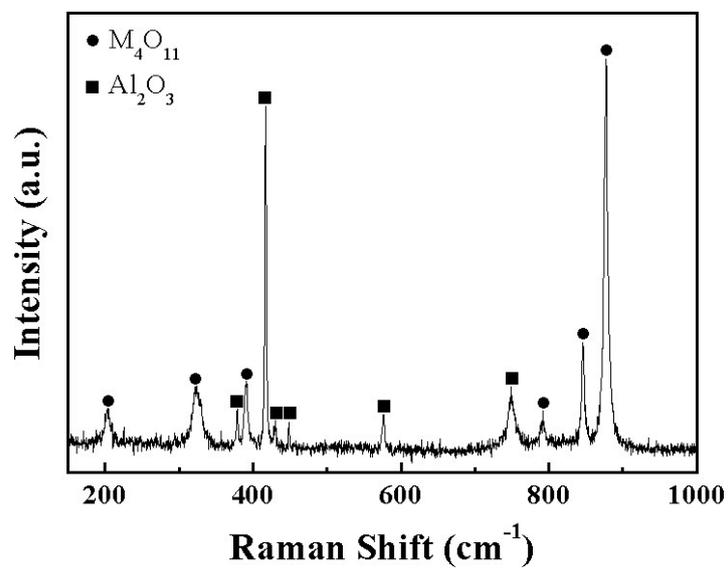
**Figure S5.** Raman spectrum of the small black particles shown in Figure 6c of the main text. Peaks marked with ● and ■ correspond to Mo<sub>4</sub>O<sub>11</sub> and Al<sub>2</sub>O<sub>3</sub>, respectively.
