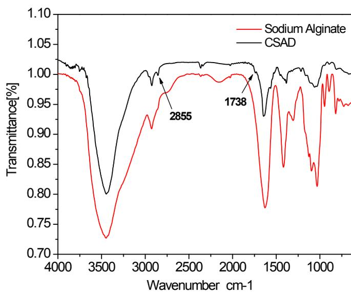
**Fig. S1** FTIR spectra of the reference sodium alginate and CSAD
