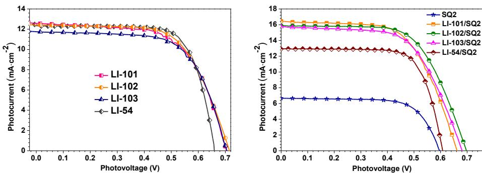
**Figure S2.**  $J$ - $V$  characteristics of DSCs based on single dyes with CDCA (5 mM) and co-sensitizers without CDCA measured at simulated  $100 \text{ mWcm}^{-2}$  AM1.5 conditions.
