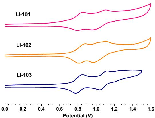
**Figure S1.** Cyclic voltammograms of sensitizers in  $\text{CH}_2\text{Cl}_2$ .
