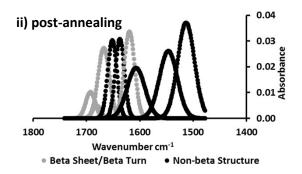
Example data: Comparison of recombinant silk films, nh-15mer, nh-15mer-R5, 15mer-ch, R5-15mer-ch, before and after the methanol annealing process with respect to the changes in protein secondary structure.
