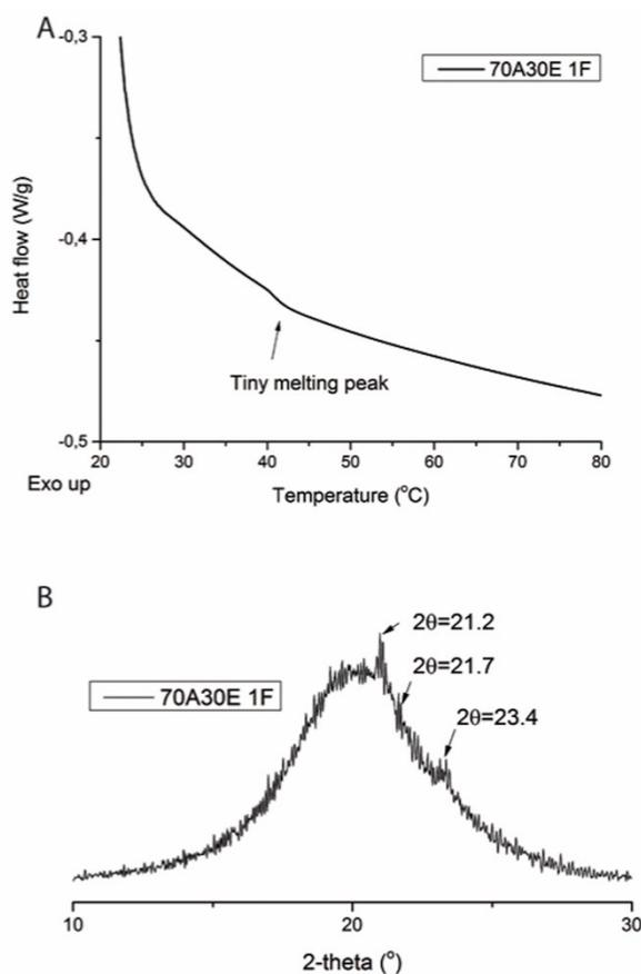
Figure S3: A) DSC thermogram (1<sup>st</sup> heating run) and B) X-Ray Diffraction (XRD) pattern of 70A30E 1F LED-cured film.
