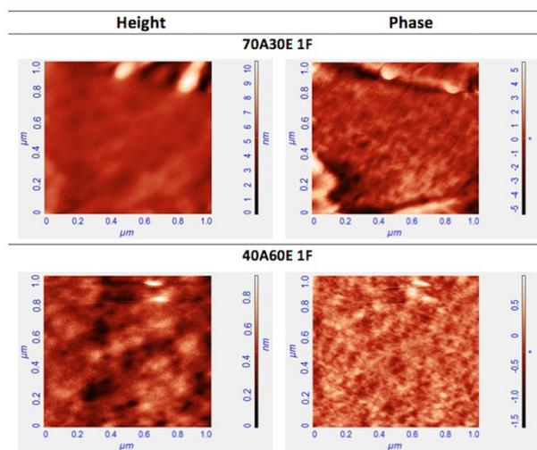
Figure S2. AFM height and phase images ( $1 \times 1 \mu\text{m}^2$ ) of crystals-free areas for 70A30E 1 F and 40A60E 1 F coatings.
