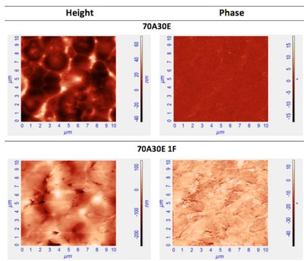
Figure S4. AFM height and phase images ( $10 \times 10 \mu\text{m}^2$ ) of surface in contact with substrate for 70A30E and 70A30E 1 F coatings.
