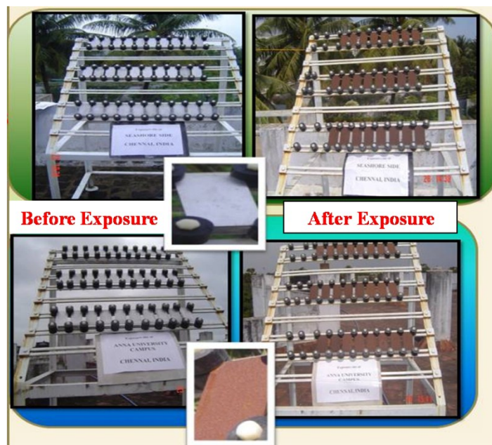
Fig. S1 Photographs of various steels in the exposure rack at the exposure site Chennai
