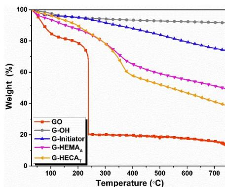
**Figure S1.** TGA thermograms of GO, G-OH, G-Initiator, G-HEMA<sub>A</sub> and G-HECA<sub>T</sub>.
