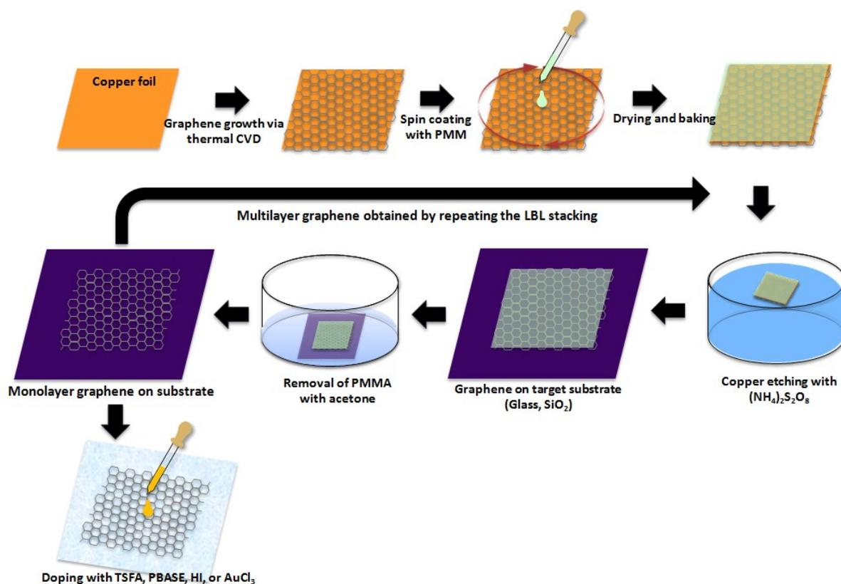
**Figure S1.** Schematic illustration of the LBL transfer and stacking of CVD-grown graphene. The processes can be divided into three main steps: (1) PMMA-assisted transfer onto the target substrate, (2) LBL stacking via the repetition of step (1) to achieve the desired number of graphene layers, and (3) chemical doping with the desired dopants.
