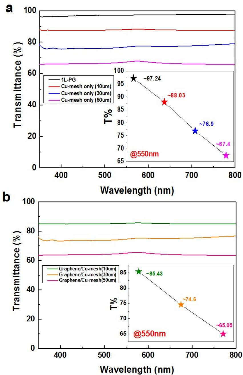
**Figure S6.** The transparency of (a) pristine graphene film and Cu mesh only with various grid widths of 10, 30, and 50  $\mu\text{m}$ ; (b) hybrid electrode composed of doped graphene and Cu mesh with various grid widths.
