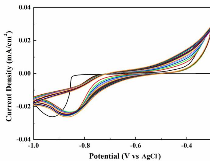
**Fig. S1.** Cyclic voltammograms during the deposition of the Co-P film using the potential cycling method.
