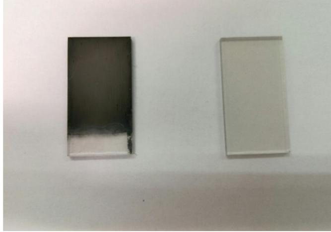
**Fig. S2.** Photographs of the Co-P/FTO (left) and blank FTO (right)
