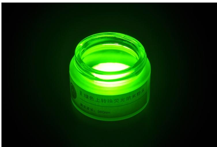
**Figure S8.** The image of NaYF<sub>4</sub>:Yb,Er UCNCs excited by a 980 nm NIR laser in a dark field.
