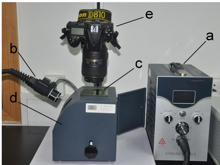
**Figure S7.** The imaging setup: (a) 980 nm NIR laser, (b) beam expander, (c) optical filter, (d) observation box, and (e) digital camera.
