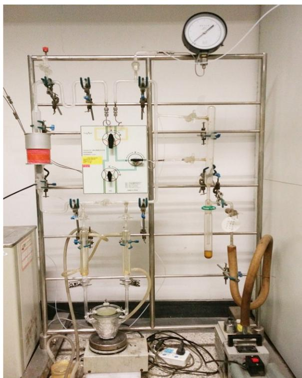
**Figure S2.** The hydrogen plant of photocatalytic experiment.
