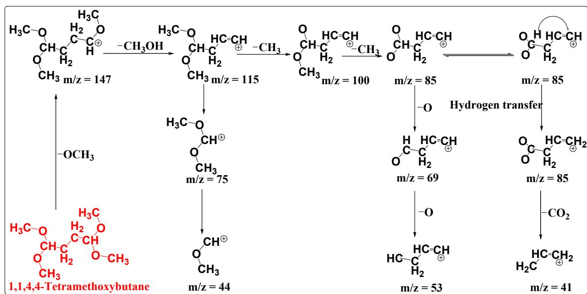
**Figure S4** Proposed reaction pathways for the dissociation of 1,1,4,4-tetramethoxybutane in the mass spectrometer.
