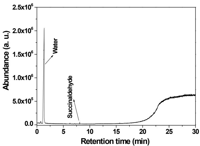
**Figure S1** GC-MS spectrum for acid-catalyzed conversion of furan in water. Reaction conditions: residence time: 20 min; furan: 3 g, water: 100 ml; catalyst: A70, 3 g; stirring rate: 350 rpm; pressure: autogenous vapor pressure.
