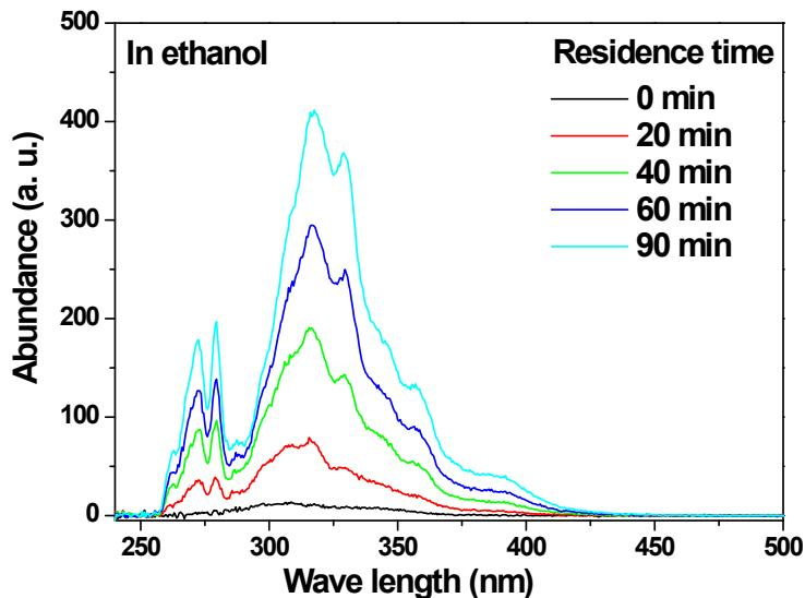
**Figure S7** Constant energy ( $- 2800 \text{ cm}^{-1}$ ) synchronous spectra for determination of the soluble polymer formed in acid-catalyzed conversion of furan in ethanol. Reaction conditions:  $T = 170^\circ\text{C}$ ; furan: 3 g, ethanol: 100 ml; catalyst: A70, 3 g; stirring rate: 350 rpm; pressure: autogenous vapor pressure. Residence time of 0 min means the reaction temperature just reached the required temperature in 10 to 14 min.
