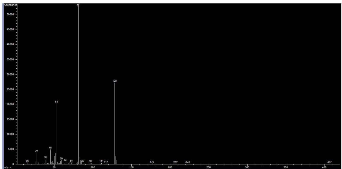
**Figure S8** Mass spectrum for furfuryl methyl sulfide.
