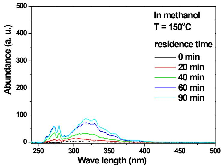
**Figure S5** Constant energy ( $- 2800 \text{ cm}^{-1}$ ) synchronous spectra for determination of the soluble polymer formed in acid-catalyzed conversion of furan in methanol. Reaction conditions:  $T = 150^\circ\text{C}$ ; furan: 3 g, methanol: 100 ml; catalyst: A70, 3 g; stirring rate: 350 rpm; pressure: autogenous vapor pressure.
