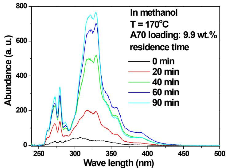
**Figure S6** Constant energy ( $-2800 \text{ cm}^{-1}$ ) synchronous spectra for determination of the soluble polymer formed in acid-catalyzed conversion of furan in methanol. Reaction conditions: furan: 3 g, methanol: 100 ml; stirring rate: 350 rpm; pressure: autogenous vapor pressure.
