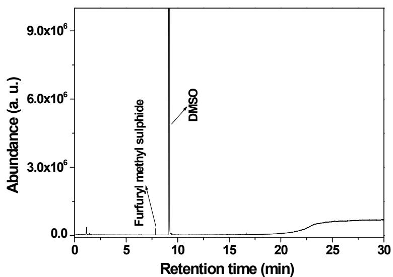
**Figure S9** GC-MS spectrum for acid-catalyzed conversion of furan in DMSO. Reaction conditions: residence time: 20 min; furan: 3 g, methanol: 100 ml; catalyst: A70, 3 g; stirring rate: 350 rpm; pressure: autogenous vapor pressure.
