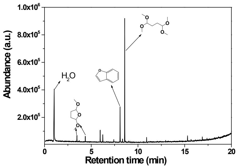
**Figure S2** GC-MS spectrum for acid-catalyzed conversion of furan in methanol. Reaction conditions: residence time: 20 min; furan: 3 g, methanol: 100 ml; catalyst: A70, 3 g; stirring rate: 350 rpm; pressure: autogenous vapor pressure.
