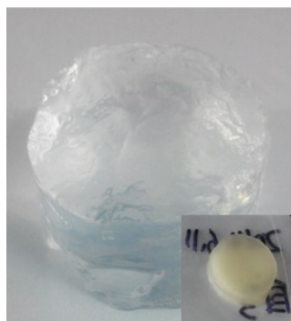
Figure S1. A typical photograph of HAG2% after equilibrium swelling in water (The inset shows the original gel just obtained after polymerization, before drying).
