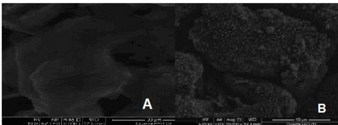
The figure shows the SEM of carbon paste electrode (CPE) (A) and AuCPE (B). The differences are observed in the surface structure of the two electrodes. For CPE, the surface appears as irregularly shaped graphite flakes and separated layers. For AuCPE surface, the nanoparticles appear at different elevations. Moreover, a random distribution and interstices among the nanoparticles were observed in SEM image of the AuCPE producing large surface area.
