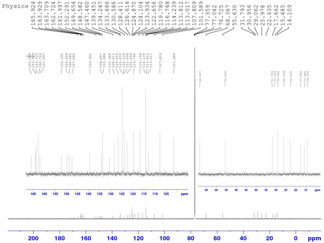
Figure S2: <sup>13</sup>C NMR spectra of compounds GK5 recorded on Bruker Avance AV- III 400 MHz NMR spectrometer.
