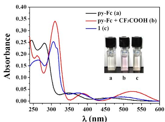
**Figure S1.** UV-Vis absorption spectra of py-Fc (a), py-Fc +  $\text{CF}_3\text{COOH}$  (b), and **1** (c) (10  $\mu\text{M}$ ) in  $\text{CH}_3\text{OH}$ .
