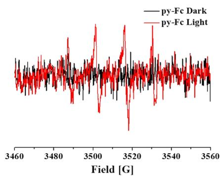
**Figure S4.** EPR signals of py-Fc (1 mM) and DMPO (50 mM) in air-saturated PBS/ $\text{CH}_3\text{CN}$  (1:1) in the dark and upon irradiation (> 400 nm) for 2 min.
