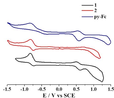
**Figure S2.** Cyclic voltammograms of **1**, **2**, and py-Fc in  $\text{CH}_3\text{OH}$  (0.1 M  $\text{Bu}_4\text{NPF}_6$ , scan rate 50  $\text{mV s}^{-1}$ ).
