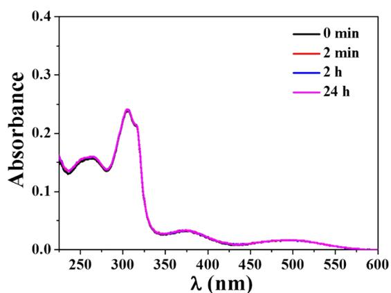
**Figure S3.** UV-Vis absorption spectra of **1** (10  $\mu$ M) in  $\text{CH}_3\text{OH}$  standing in the dark for 24 h.
