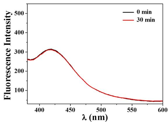
**Figure S6.** Fluorescence intensity changes of an aqueous solution containing 1 mM TA, 2 mM NaOH, 100  $\mu$ M **1** and 50 mM KI before and after irradiation at 470 nm (LED light source) for 30 min.
