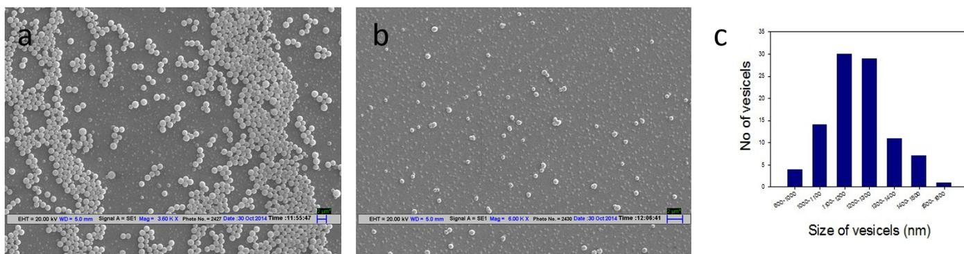
**Figure S9:** (a) SEM image of 1 mM solution of **M3** in CH<sub>3</sub>OH, scale bar 2 μm (b) SEM image of 0.1 mM solution of **M3** in CH<sub>3</sub>OH, scale bar 2 μm (c) Histogram showing the size distribution of vesicles.
