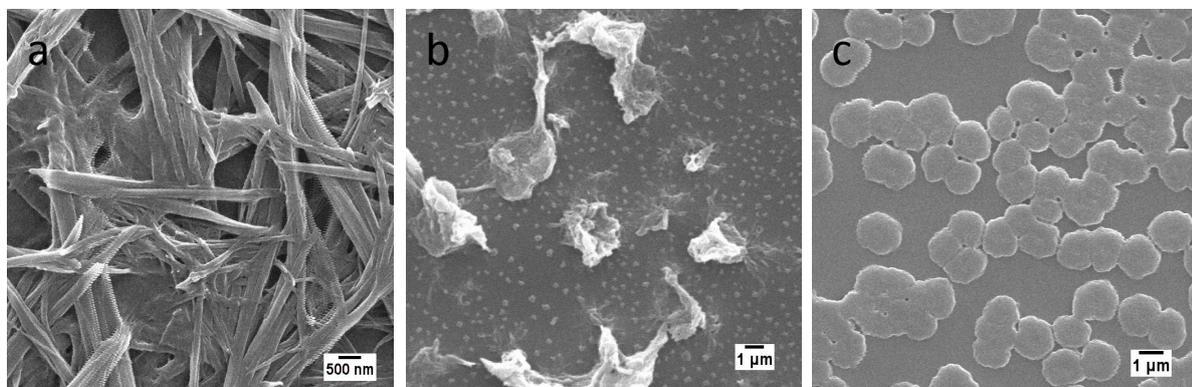
**Figure S1:** SEM image of 1 mM solution of **M1** in (a) Ethylacetate (b) Chloroform: Methanol (1:1) (c) isopropanol
