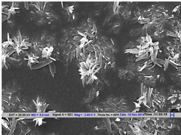
**Figure S7:** SEM image of **A1** (1 mM, CH<sub>3</sub>OH)
