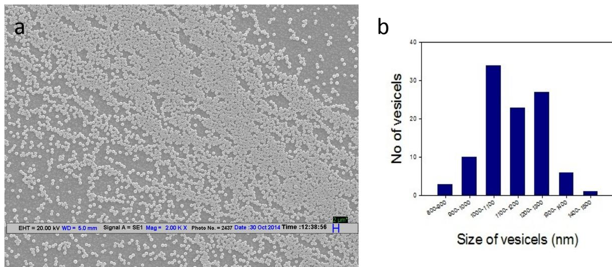
**Figure S12:** (a) Low magnification SEM image of **M4**, scale bar 2  $\mu\text{m}$  (b) Histogram showing the size distribution of vesicles.
