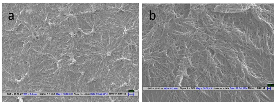
**Figure S5:** SEM image of (a) 0.1 mM solution of **M2** in methanol scale bar 1 μm and (b) enlarged image, scale bar 200 nm.
