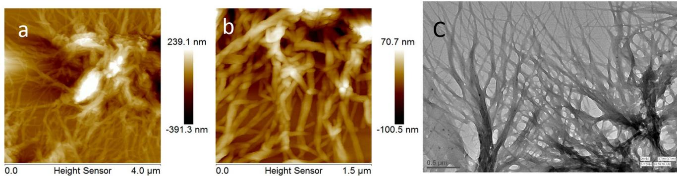
**Figure S6:** AFM images of 1 mM solution of **M2** in methanol (a) low magnification (b) high magnification (c) HRTEM image of **M2** (1 mM, methanol)
