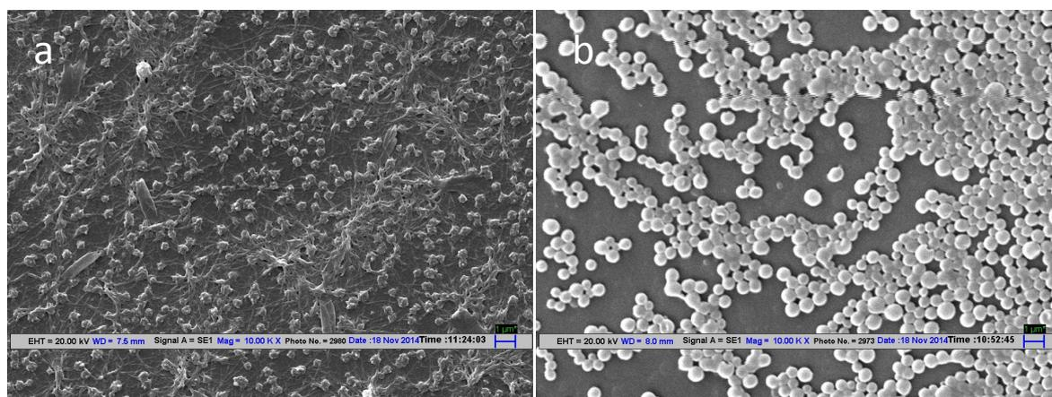
**Figure 11:** SEM images of 1 mM solution of (a) **A2** scale bar 1 μm (b) **A4** scale bar 1 μm. Both samples are prepared in methanol.
