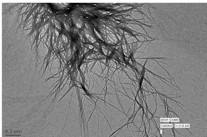
**Figure S4:** HR-TEM image of 1 mM solution of **M1** in methanol low magnification (Scale bar 500 nm).
