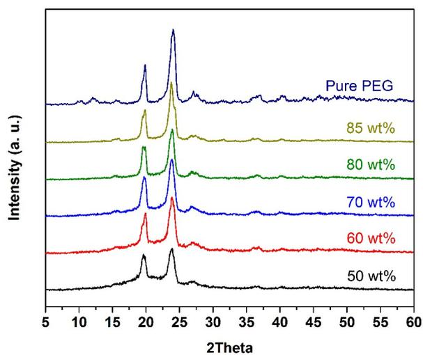
**Fig S6.** XRD patterns of PEG-6000@NP-B PCMs with various PEG mass fractions.
