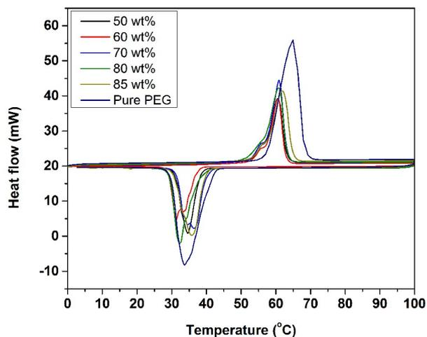
**Fig S8.** The DSC curves of PEG-6000@NP-B PCMs composites with various PEG mass fractions.
