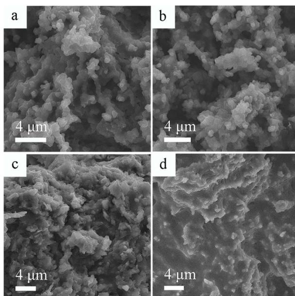
**Fig S4.** SEM images of PEG@NP-B with different mass fraction: (a) 50 wt%, (b) 60 wt%, (c) 70 wt% and (d) 80 wt%.
