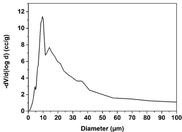
**Fig S2.** Pore size distribution curve of NP-B tested by mercury porosimetry.
