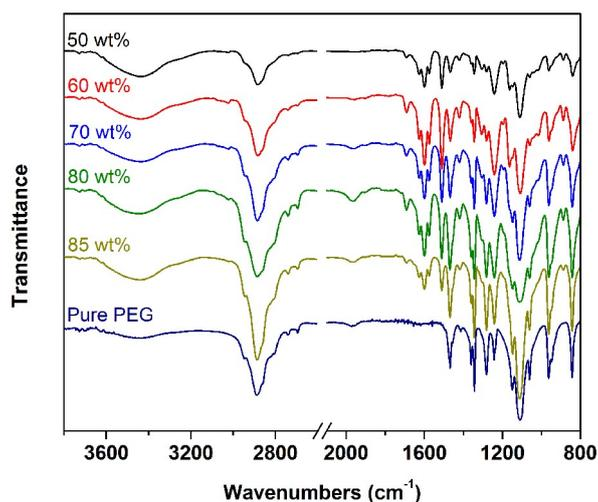
**Fig S7.** FT-IR spectrums of PEG-6000@NP-B PCMs with various PEG mass fractions.
