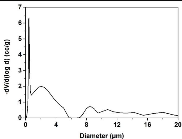
**Fig S1.** Pore size distribution curve of NP-A tested by mercury porosimetry.
