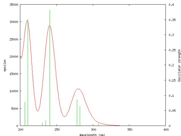
**Fig. 16S.** Calculated electronic absorption spectrum of **HL** [using conductor-like polarizable continuum model (CPCM) in ethanol; basis set, 6-31G(d-p)].
