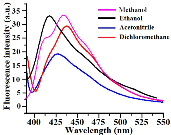
**Fig.12S.** Fluorescence spectra of complex **2** recorded in acetonitrile (blue line), methanol (pink line), ethanol (black line) and dichloromethane (red line).
