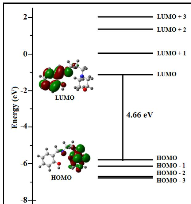
**Fig.41S.** Calculated molecular orbital energy level diagram of **HL** [B3LYPfunctional; basis set 6-31G(d-p), using conductor-like polarizable continuum model (CPCM) in methanol].
