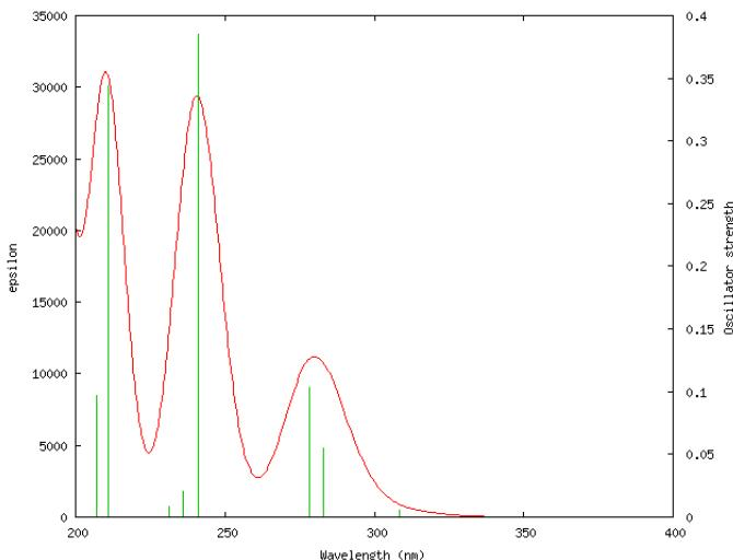
**Fig. 18S.** Calculated electronic absorption spectrum of **HL** [using conductor-like polarizable continuum model (CPCM) in dichloromethane; basis set, 6-31G(d-p)].
