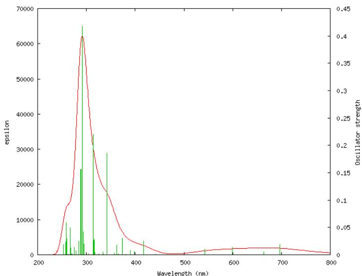
**Fig. 25S.** Calculated electronic absorption spectrum of **1** [using conductor-like polarizable continuum model (CPCM) in acetonitrile; basis set, LanL2DZ].
