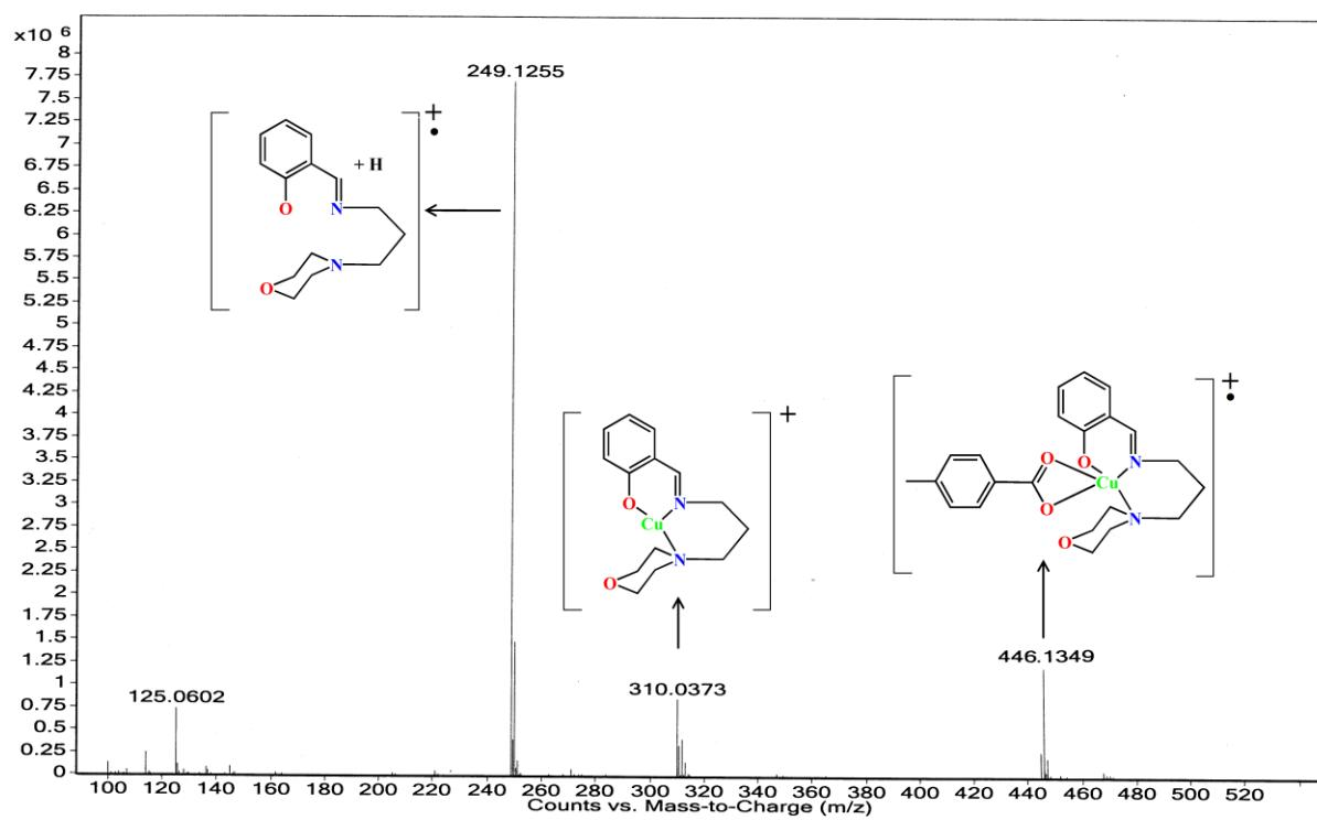
**Fig.4S.** ESI mass spectra of complex **2** recorded in methanol.
