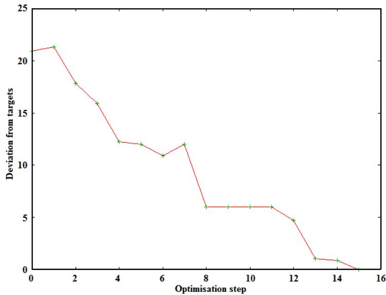
**Fig.45S.** Deviation from target vs. optimization step of HL [using conductor-like polarizable continuum model (CPCM) in methanol; basis set, 6-31G(d-p)].
