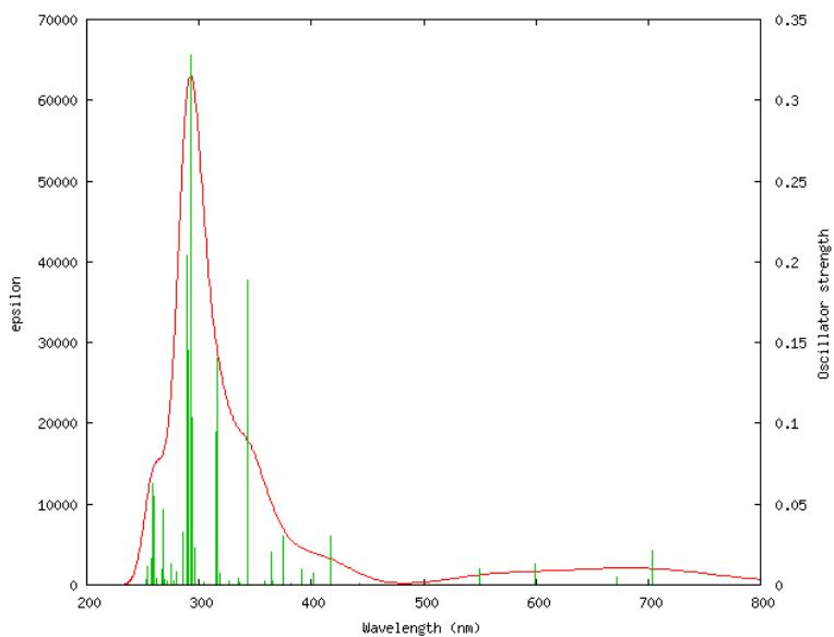
**Fig. 26S.** Calculated electronic absorption spectrum of **1** [using conductor-like polarizable continuum model (CPCM) in dichloromethane; basis set, LanL2DZ].
