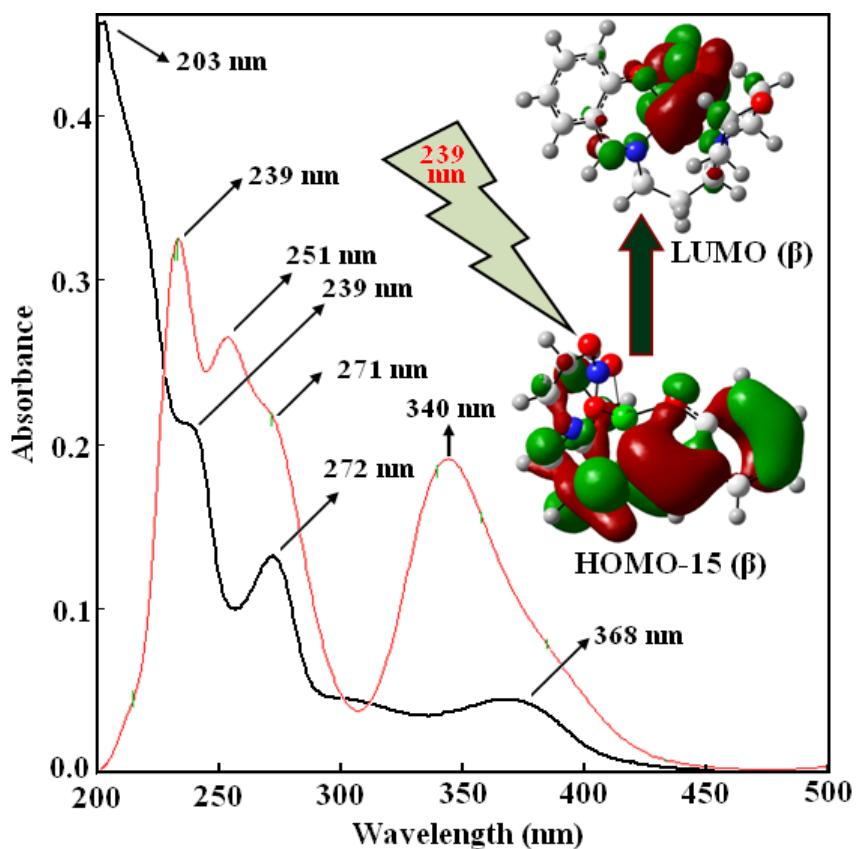
**Fig.36S.** Theoretical and experimental absorbance spectra of model compound.
