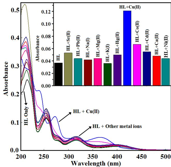
**Fig.33S.** UV-Vis spectra of 3 ml 0.98 $\mu$ M methanolic solution of HL upon addition of 150  $\mu$ l 25.66  $\mu$ M methanolic solution of various metal ions keeping the anion fixed (nitrate in the present case) [inset bar diagram represent the absorbance at 272 nm].
