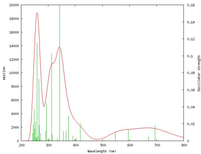
**Fig. 27S.** Calculated electronic absorption spectrum of **2** [using conductor-like polarizable continuum model (CPCM) in ethanol; basis set, LanL2DZ].
