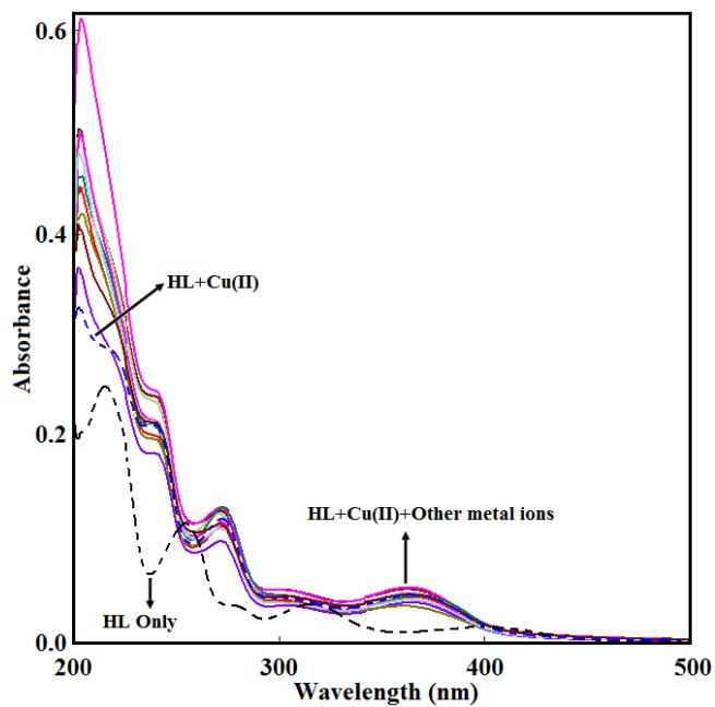
**Fig.34S.** UV-Vis spectra of adduct containing 3 ml 0.98 $\mu$ M methanolic solution of HL and 150  $\mu$ l 25.66  $\mu$ M methanolic solution of Cu(II) ion upon addition of 150  $\mu$ l 25.66  $\mu$ M methanolic solution of different metal ions keeping the anionic unit fixed (nitrate in the present case).
