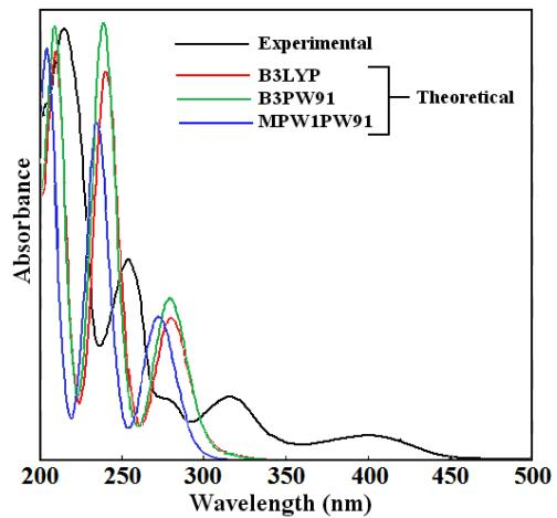
**Fig. 32S.** Experimental (black line) and theoretical (red, green and blue line, using B3LYP, B3PW91, MPW1PW91 functionals, respectively) electronic spectra of HL.
