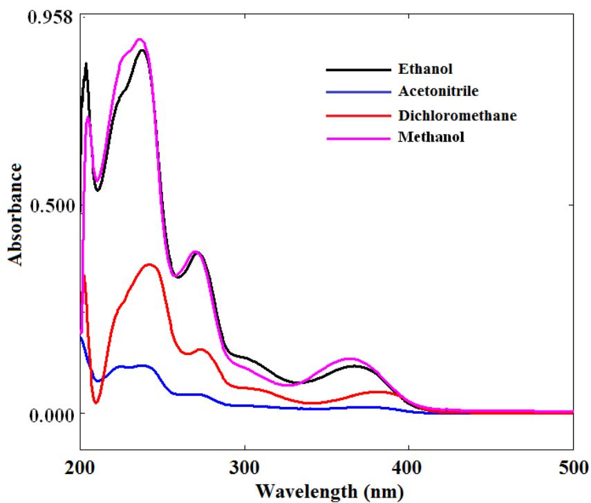
**Fig.7S.** Electronic absorption spectra of complex **2** recorded in acetonitrile (blue line), methanol (pink line), ethanol (black line) and dichloromethane (red line).
