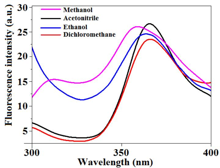
**Fig.8S.** Fluorescence spectra of **HL** recorded in acetonitrile (black line), methanol (pink line), ethanol (blue line) and dichloromethane (red line) [ $\lambda_{\text{ex}} = 254$  nm, for all solvents].
