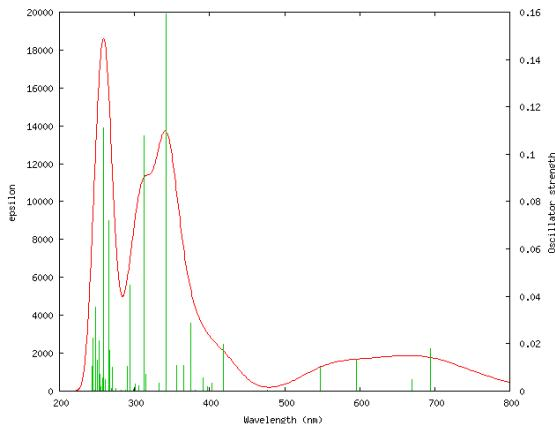
**Fig. 28S.** Calculated electronic absorption spectrum of **2** [using conductor-like polarizable continuum model (CPCM) in acetonitrile; basis set, LanL2DZ].
