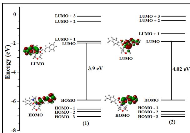
**Fig.22S.** Calculated  $\alpha$  molecular orbital energy level diagram of **1** and **2** [B3LYP functional; basis set LanL2DZ; using conductor-like polarizable continuum model (CPCM) in methanol].
