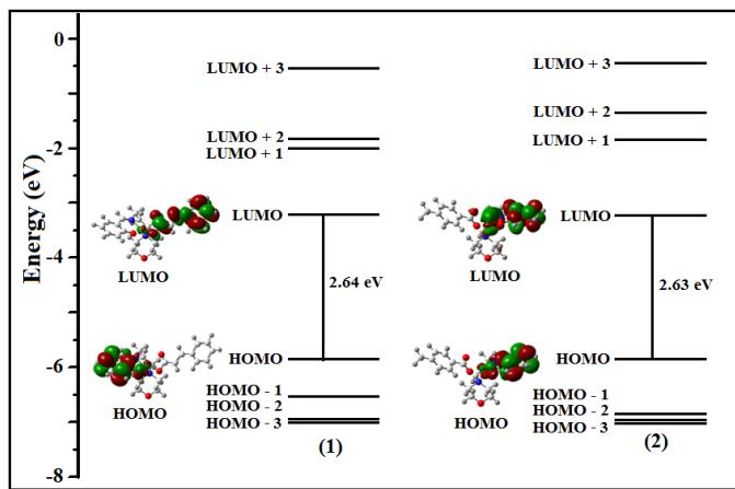
**Fig.23S.** Calculated  $\beta$  molecular orbital energy level diagram of **1** and **2** [B3LYP functional; basis set LanL2DZ, using conductor-like polarizable continuum model (CPCM) in methanol].
