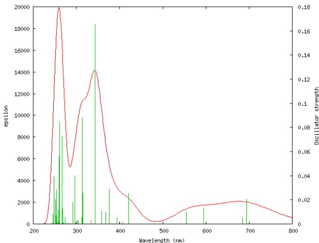
**Fig. 29S.** Calculated electronic absorption spectrum of **2** [using conductor-like polarizable continuum model (CPCM) in dichloromethane; basis set, LanL2DZ].
