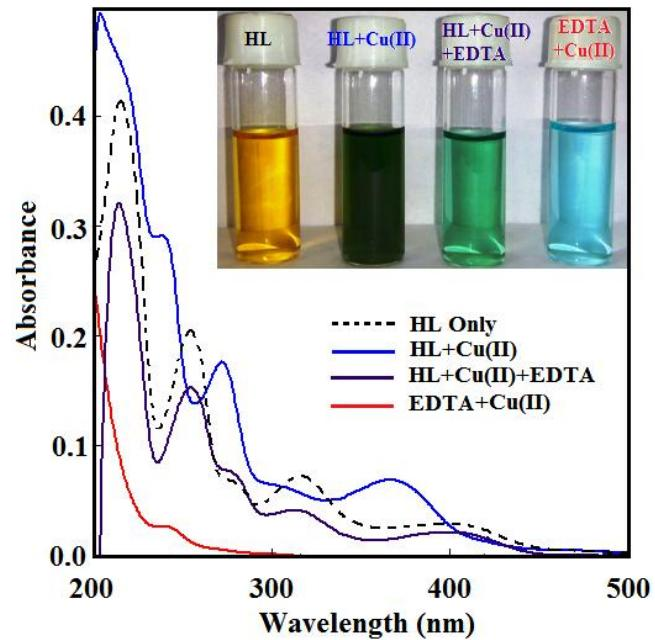
**Fig. 35S.** UV-vis absorption spectra of HL with  $\text{Cu}(\text{NO}_3)_2 \cdot 3\text{H}_2\text{O}$ . In presence and absence of EDTA.
