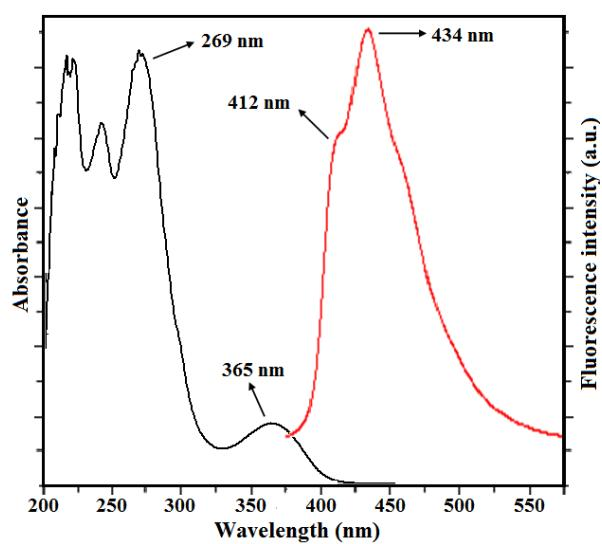
**Fig.9S.** Absorption (left) and fluorescence (right) spectra of complex **1**.
