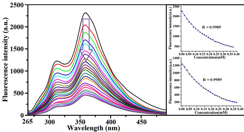
**Fig.38S.** Fluorescence of 3 ml 0.1 mM methanolic solution of HL upon gradual addition of 10 µl 5 mM methanolic solution of Cu(II) ion keeping the anion fixed (nitrate in the present case) [Inset (a) represent decrease of fluorescence intensity upon gradual addition of Cu(II) at 359nm whereas (b) represent that at 313 nm].
