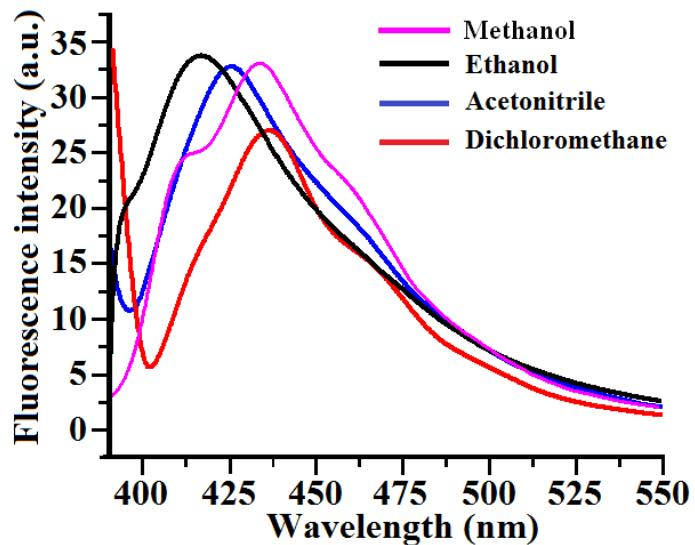
**Fig.11S.** Fluorescence spectra of complex **1** recorded in acetonitrile (blue line), methanol (pink line), ethanol (black line) and dichloromethane (red line).
