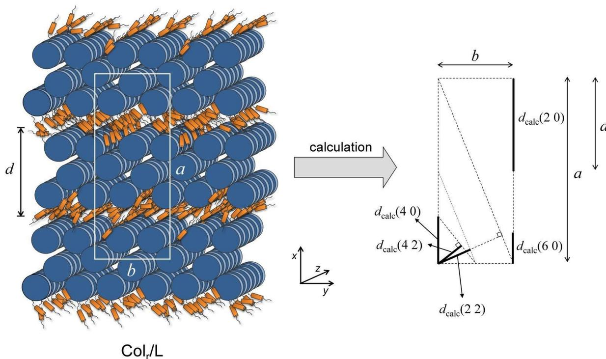
**Figure S9** Denoting the calculated diffraction spacing  $d_{\text{calc}}$  and layer spacing  $d$  within the rectangular  $p2gg$  lattice of Col<sub>r</sub>/L phase.
