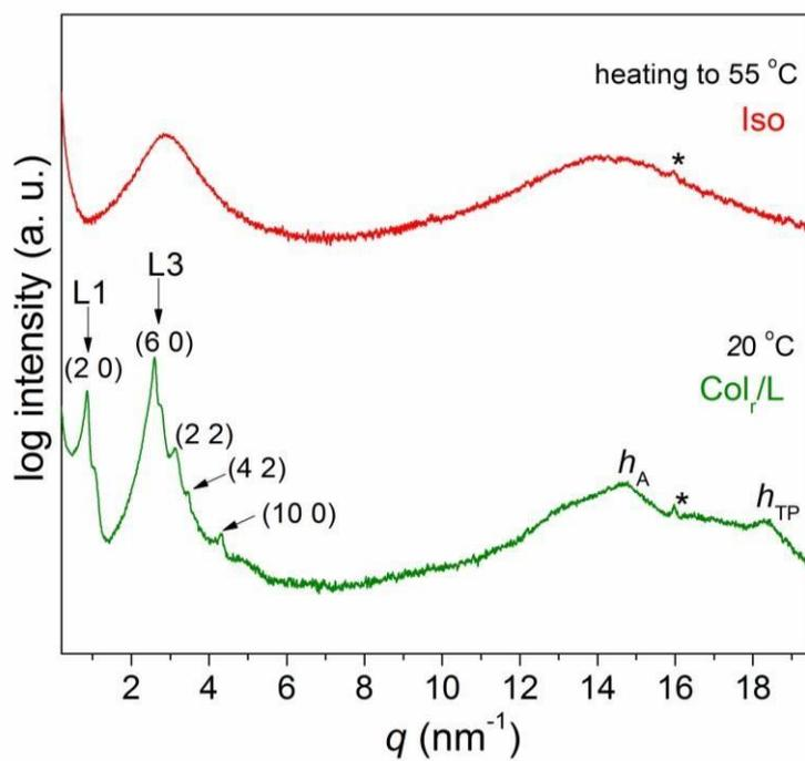
**Figure S8** Typical SAXS/WAXS profiles of TP10-AZO12. The wide-angle reflections labeled with an asterisk are from background aluminum foil.
