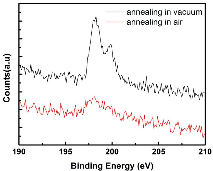
Figure S4. Cl<sub>2</sub>p core level XPS spectra of the perovskite films.
