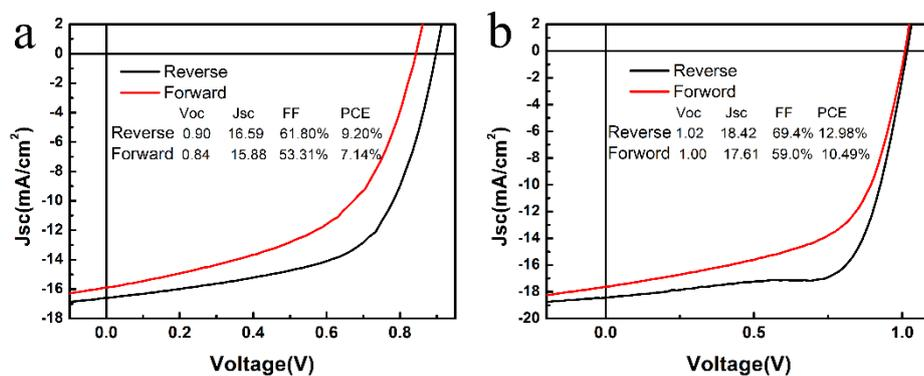
**Figure S2.** Hysteresis J-V measurements scanned in forward (red) and reverse (black) directions for devices annealed in air (a) and vacuum (b).
