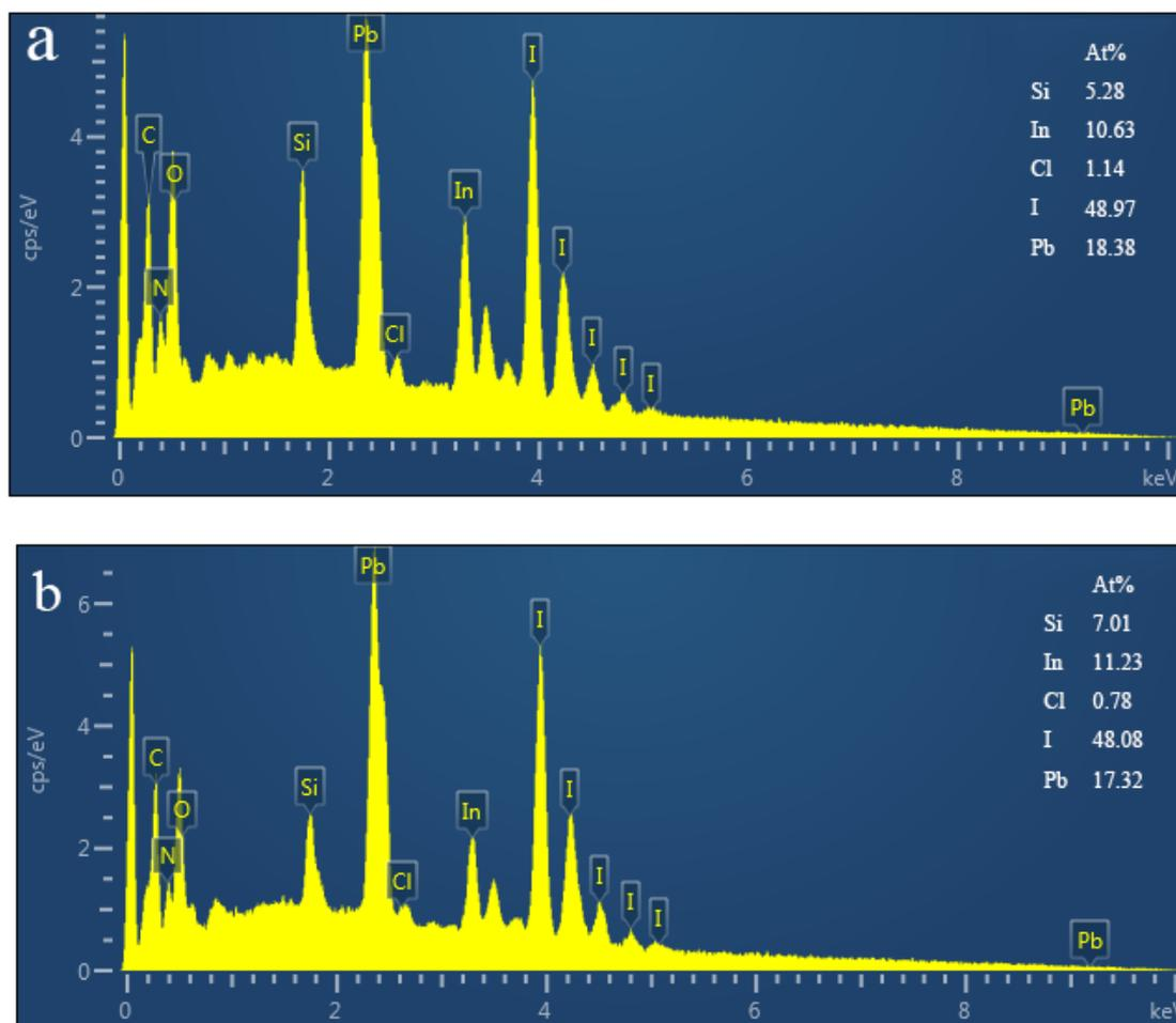
**Figure S3.** The characterization of EDS for perovskite films annealed in vacuum (a) and air (b).
