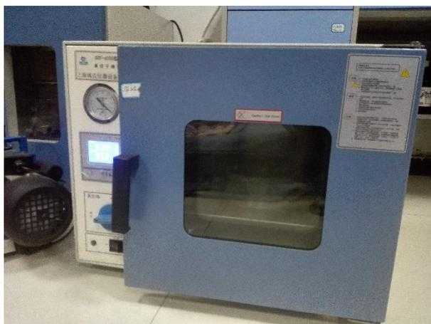
**Figure S1.** The vacuum oven for vacuum annealing.
