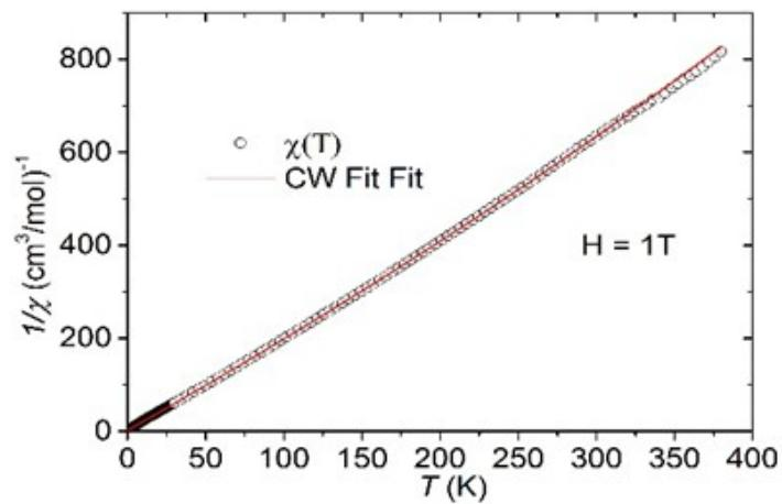
**Fig. S4**  $1/\chi$  data of compound **1** (solid line represent the Currie-Weiss fitting).
