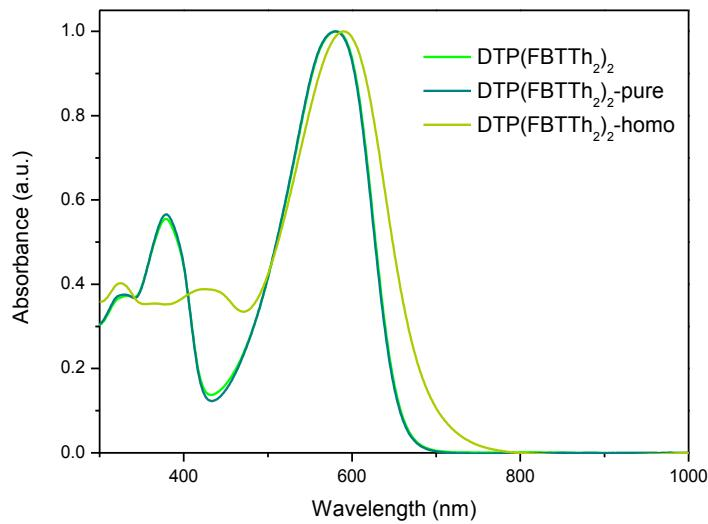
**Figure S5:** UV-Vis absorption spectra (normalized) for **DTP(FBTTh<sub>2</sub>)<sub>2</sub>**, **DTP(FBTTh<sub>2</sub>)<sub>2</sub>-pure** and **DTP(FBTTh<sub>2</sub>)<sub>2</sub>-homo** in CHCl<sub>3</sub>.
