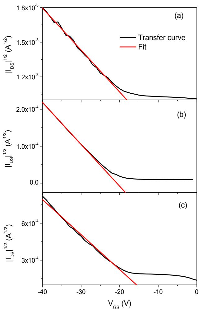
**Figure S3:** FET transfer characteristics for **CPDT(FBTTh<sub>2</sub>)<sub>2</sub>** (a), **DTP(FBTTh<sub>2</sub>)<sub>2</sub>-pure** (b), and **TT(FBTTh<sub>2</sub>)<sub>2</sub>** (c). The lines used to fit the mobilities in the saturation regime ( $V_{DS} = -40$  V) are shown in red.
