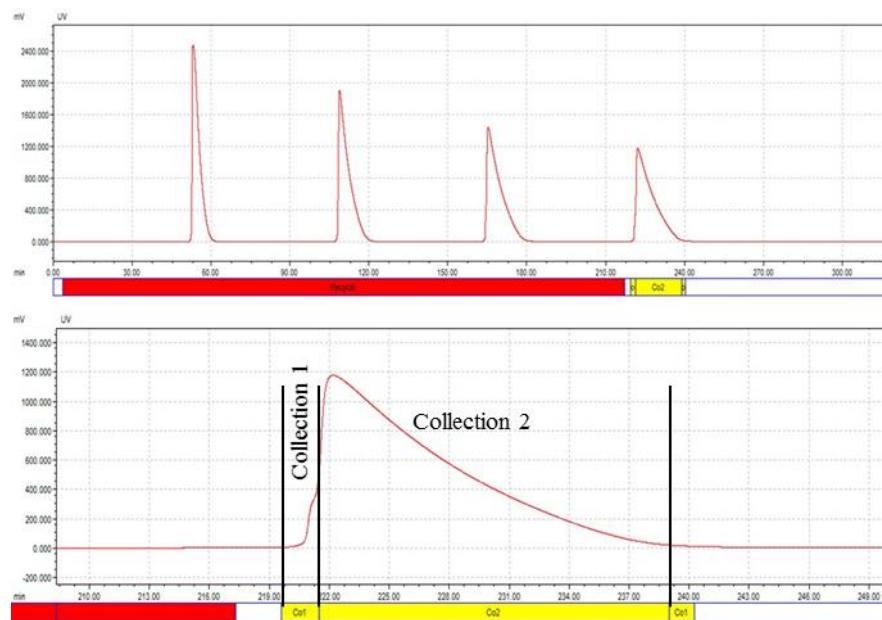
**Figure S4:** Prep-SEC trace for the purification of **DTP(FBTTh<sub>2</sub>)<sub>2</sub>**. **DTP(FBTTh<sub>2</sub>)<sub>2</sub>-homo** can be separated as the first collection.
