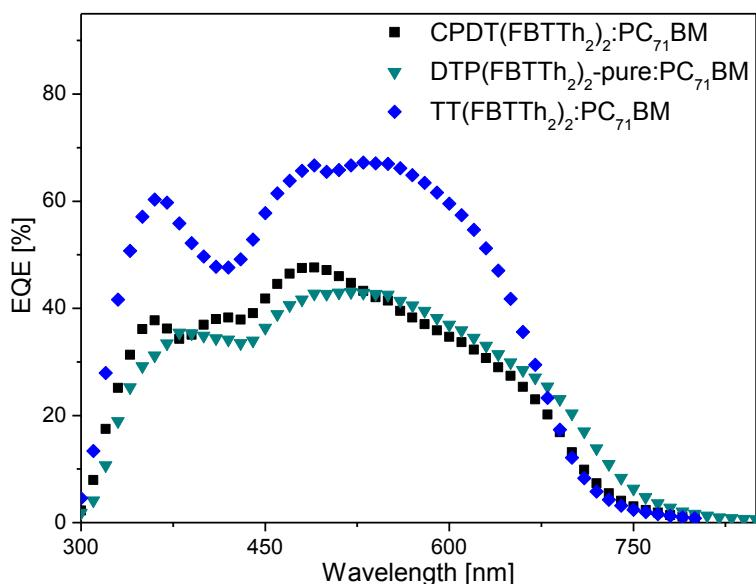
**Figure S2:** EQE spectra of the optimal devices prepared from the three small molecules.
