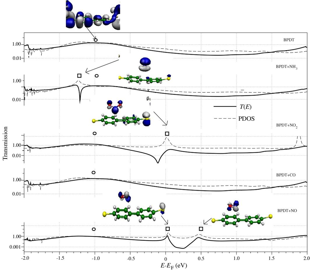
Figure S2: The transmission coefficients and PDOS of BPDT-Au junction with and without gas adsorption. The PDOS and transmission peaks associated with the HOMO of isolated nucleobases (circle) and molecular orbitals of gas molecules (square) are identified.
