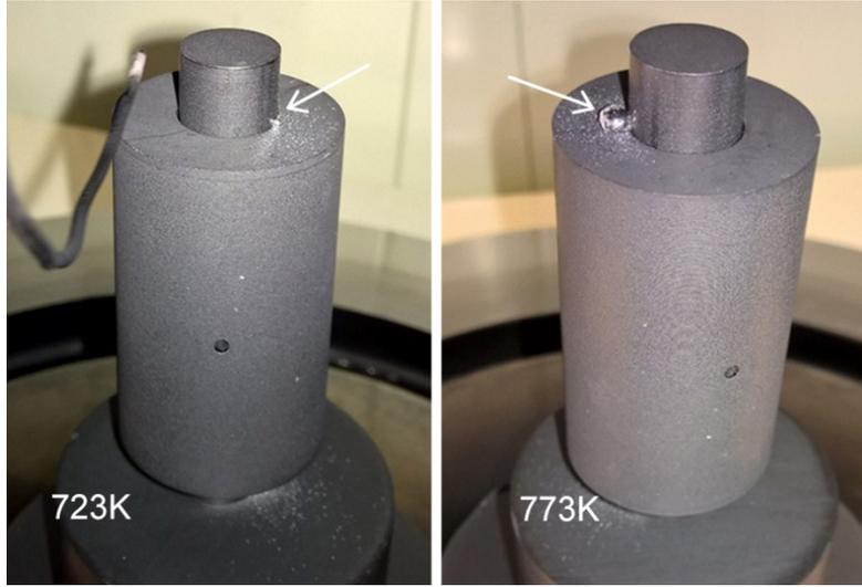
**Fig. S6** Spilled droplets squeezed out of graphite die after SPS sintering at 723 K (left) and 773 K (right).
