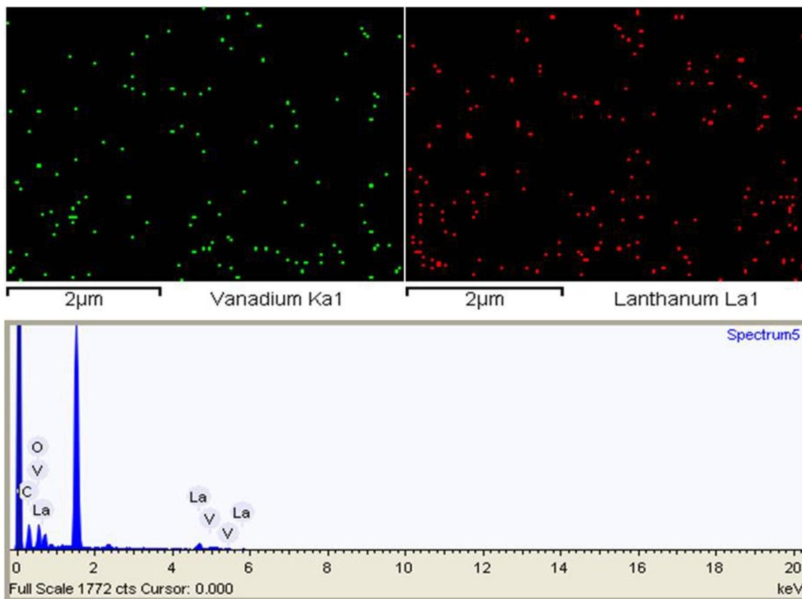
Figure S1: Energy dispersive X-ray spectroscopy (EDX) analysis of PEGylated polymer capsules encapsulating  $\text{LaVO}_4:\text{Tb}^{3+}$  nanoparticles.
