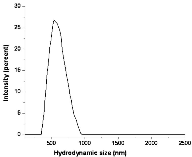
Figure S2. Dynamic light scattering measurement of PEGylated polymer capsules encapsulating LaVO<sub>4</sub>:Tb<sup>3+</sup> nanoparticles.
