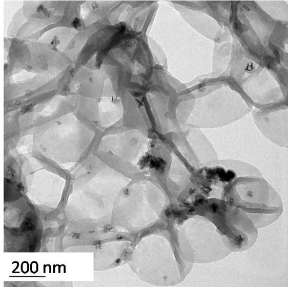
Figure S3. TEM image of PEGylated polymer capsules encapsulating  $\text{LaVO}_4:\text{Tb}^{3+}$  nanoparticles (Images are acquired after six months of synthesis of capsules to study the stability)
