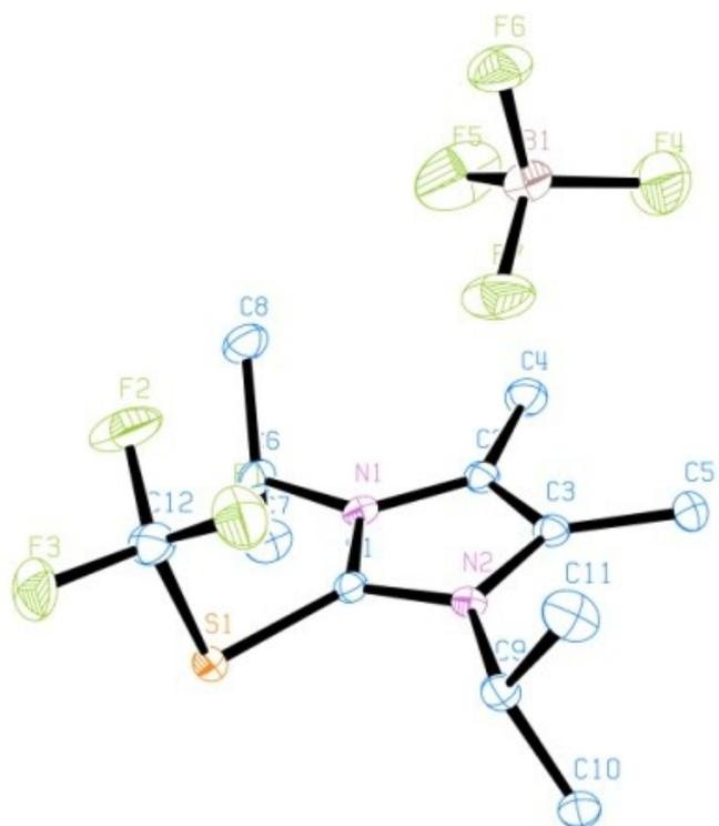
Figure1. ORTEP drawing of the X-ray structure of **4c**. Hydrogen atoms are omitted for clarity and ellipsoids displayed at 50% probability. Selected bond distances (Å), angles [deg] and torsional Angles[deg] in **4c**, C1–S1, 1.732 (2); S1–C12, 1.808 (3); F1–C12, 1.323(3); F2–C12, 1.342(3); F3–C12, 1.333(3); C1–S1–C12, 97.48 (11); C12–S1–C1–N1, –93.99 (19); C12–S1–C1–N2, 89.66 (19)
