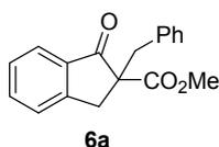
Synthesized following GP-A (0.25 mmol scale). A mixture of indanone **5** (47.5 mg, 0.25 mmol), benzylbromide (45  $\mu$ l, 0.38 mmol), **4c** (9.2 mg, 0.025 mmol) and KOH (42 mg, 0.75 mmol) in CHCl<sub>3</sub> (1.2 mL) was stirred for 1hr. Purified by SiO<sub>2</sub> gel column chromatography (acetone : n-hexane=1 : 9) to give 65.8 mg
