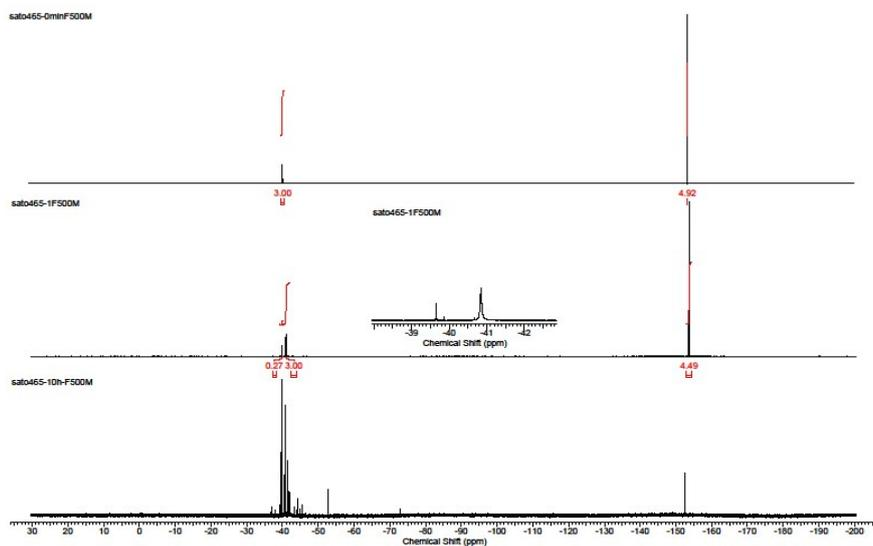
(top)  $^{19}\text{F}$  NMR spectrum of **4c**. (middle)  $^{19}\text{F}$  NMR spectrum of crude mixture for while stirring for 1h. (bottom)  $^{19}\text{F}$  NMR spectrum of crude mixture for while stirring for 10 hrs.
