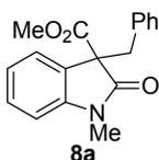
Synthesized following GP-A (0.20 mmol scale). A mixture of **7** (41.0 mg, 0.20 mmol), benzyl bromide (36  $\mu$ l, 0.30 mmol), **4c** (7.4 mg, 0.02 mmol) and KOH (34 mg, 0.60 mmol) in  $\text{CHCl}_3$  (1.0 mL) was stirred for 30 min. Purified by  $\text{SiO}_2$  gel column chromatography (EtOAc : n-hexane=1 : 2) to give 56.0 mg (95 % yield) of the title compound as a white solid.
